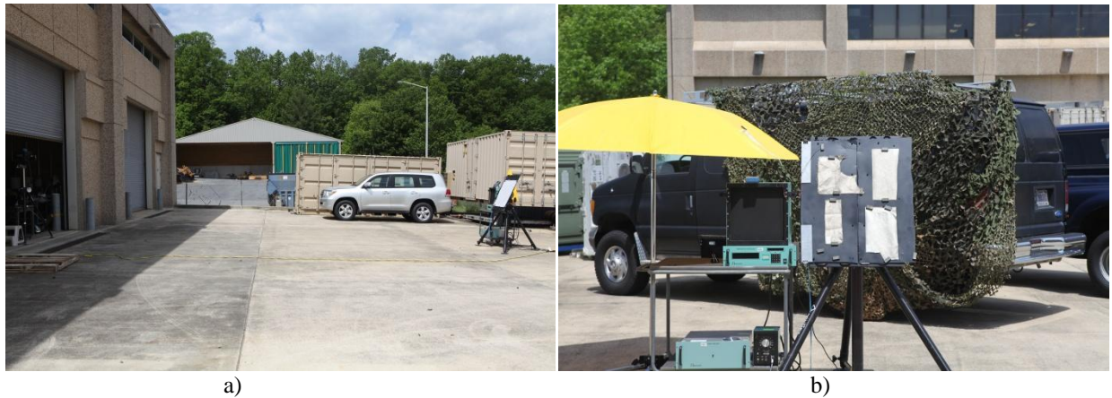
Fig. 7 a) In the polarimetric-measurement setup the LWIR polarimetric camera is located in the shadow on the left side of the photograph. b) The heated test panel has 4 sample materials attached; a calibrated black body—van with camouflage netting—is positioned in the scene and is set at a constant temperature of 37 °C. Typical test-panel temperatures ranged from 40 to 50 °C depending on the degree of solar loading.
