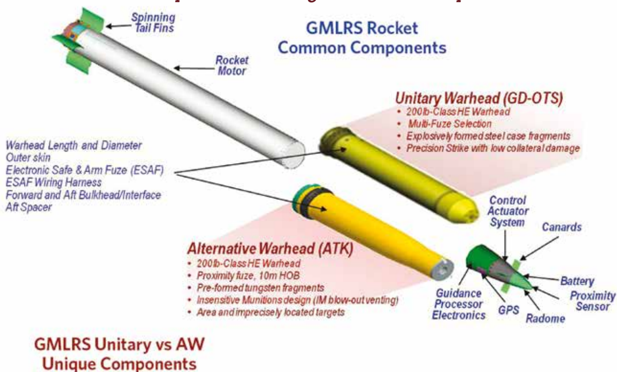
Figure 2. Guided Rocket System With Change in Warhead Only
