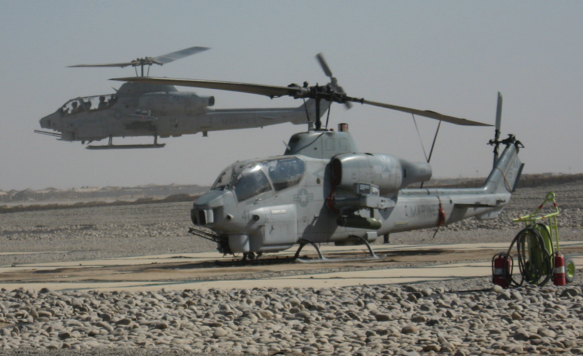
AH-1 Cobras at Forward Operating Base (FOB) Dwyer well protected by Aircraft Survivability Equipment, including Missile Warning Sensors and Countermeasure Dispensers visible here. Naval Air Systems staff photo
