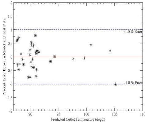
**Figure 22:** ANN-Engine model prediction of outlet temperature (°C)
