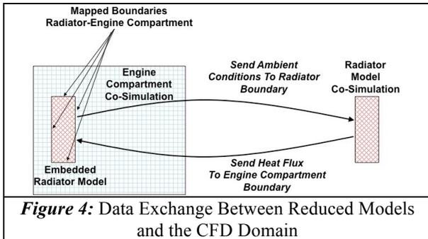
**Figure 4:** Data Exchange Between Reduced Models and the CFD Domain
