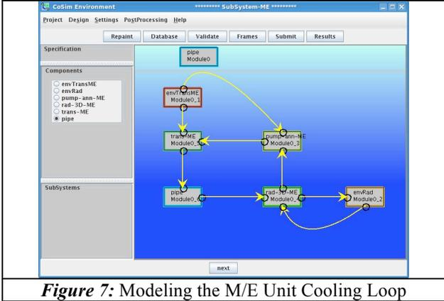
Figure 7: Modeling the M/E Unit Cooling Loop
