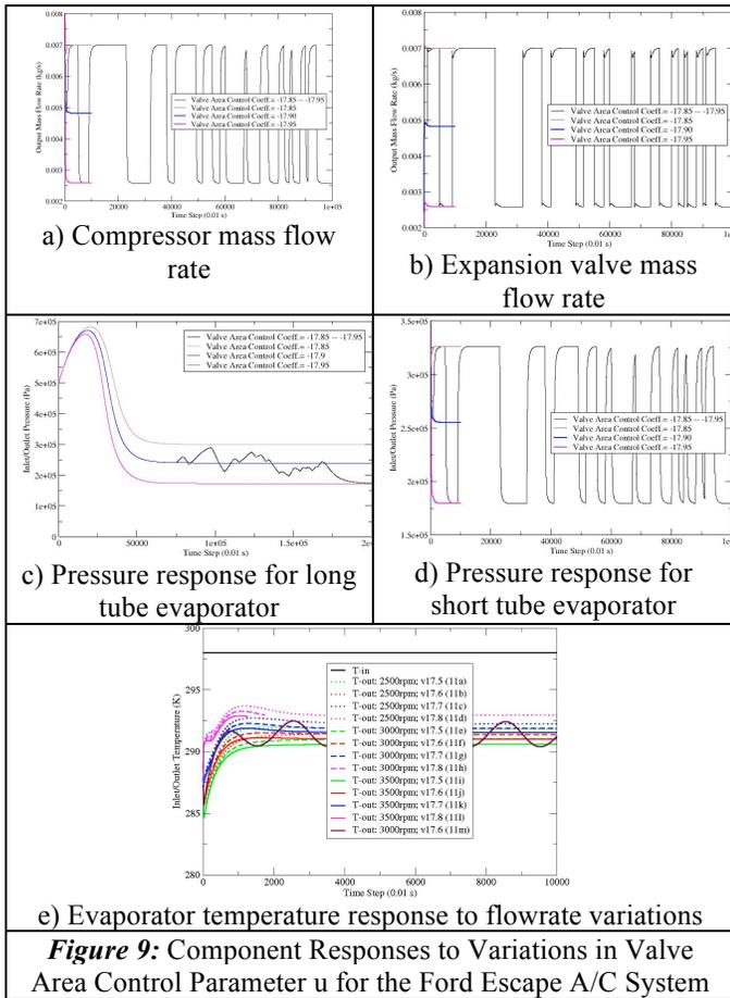
**Figure 9:** Component Responses to Variations in Valve Area Control Parameter  $u$  for the Ford Escape A/C System
