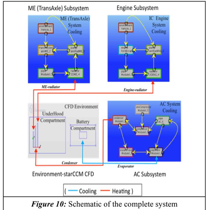
**Figure 10:** Schematic of the complete system
