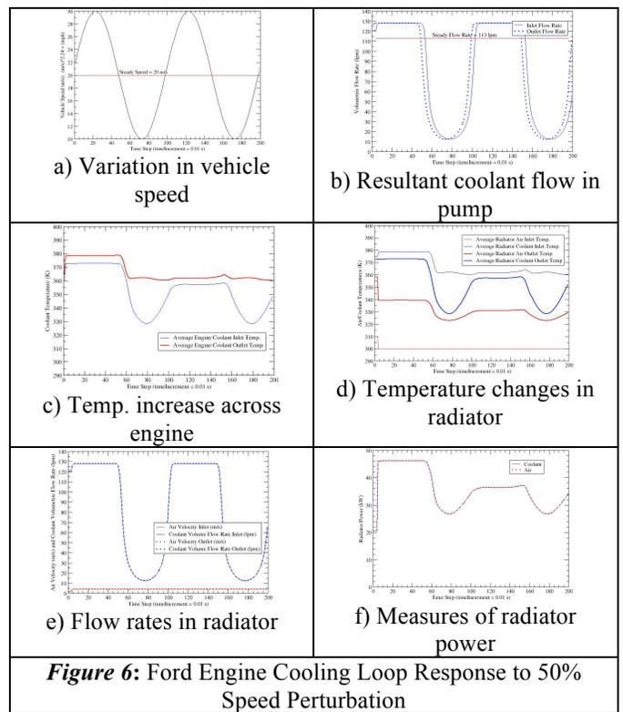
**Figure 6:** Ford Engine Cooling Loop Response to 50% Speed Perturbation
