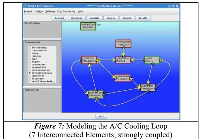
Figure 7: Modeling the A/C Cooling Loop (7 Interconnected Elements; strongly coupled)
