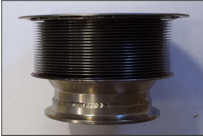
Figure 4: Example of mechanical bellows used as injecting source
