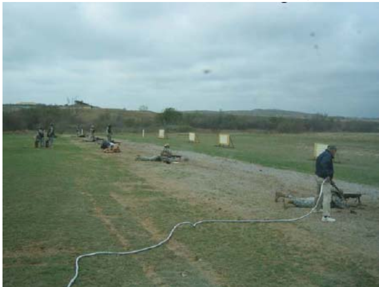
Figure 3-7. M249 5.56mm Squad Automatic Weapon (SAW). Individual soldiers fired the M249 (20-50 rounds per soldier) from prone positions from five firing positions located side-by-side. Muzzle plumes/breech plumes of one gun were measured in the breathing zone by handholding the sampling line near the breech (shown in the picture). Wind speed = 5.6 \pm 1.4 m/s.
