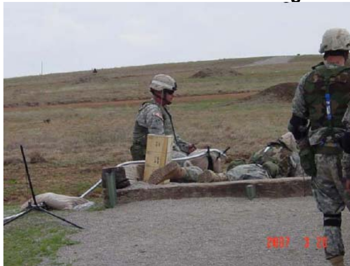
Figure 3-8. M240 7.62mm Machine Gun. Individual soldiers fired the M240 weapons (20-50 rounds per soldier) from prone positions with eight firing positions located side-by-side. The muzzle emissions/breech plumes of several individual guns (from the firing line) in the breathing zone were sampled during firing by placing the sampling line on a small tripod located just down wind of the breech (shown in the picture) and 3 meters further down wind (not shown). Wind speed = 8.1 \pm 1.6 m/s.
