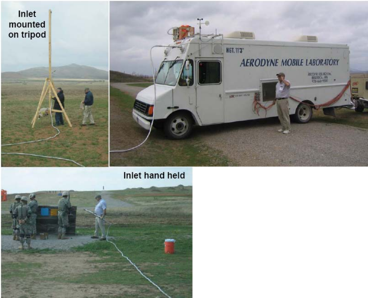
Figure 3-1. Aerodyne Mobile Laboratory and Sampling Line Deployment. The mobile laboratory was stationed within 30 meters of the weapons systems. The sampling probe was
