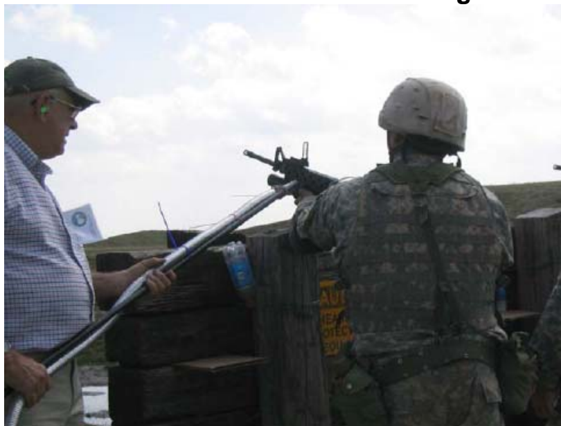
Figure 3-6. M203 Grenade Launcher. Individual soldiers fired the M203 from behind the wood posts from two side-by-side positions. Muzzle plume emissions/breech plumes were sampled in the breathing zone via a hand held sampling line (shown in the picture). Wind speed = 9.9 \pm 1.6 m/s.
