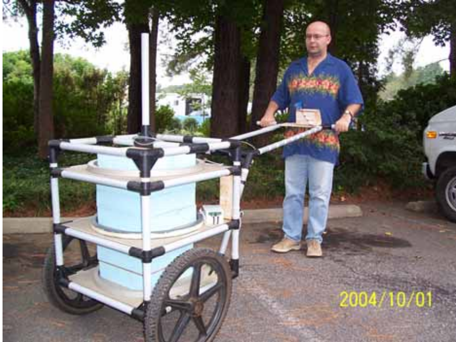
Figure 1. Original cart-mounted coaxial EMI system with 23 cm radius coils separated by 25 cm; the transmitter electronics module can be seen adjacent to the central transmitter coil, and the battery pack mounted on the cart handle. The Styrofoam (blue) blocks were inserted to reduce “drumhead” vibrations.
