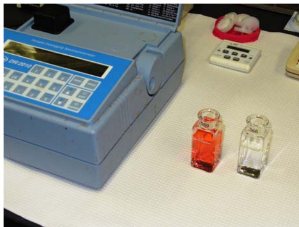
Figure 3-3. CRREL Method Color Development
