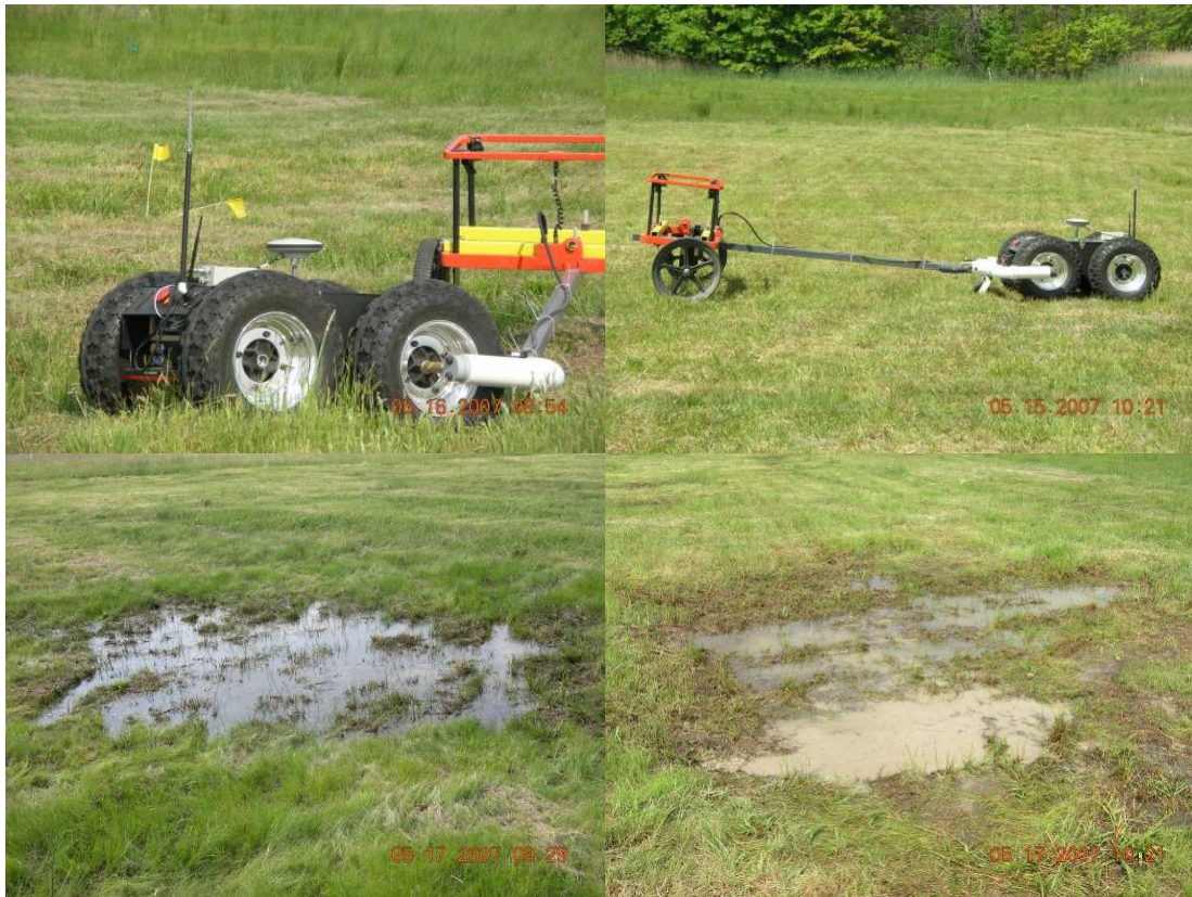
Figure 4-4: Robot-Open Field Top- Robot with EM-61 in Open Field Bottom- Water Hazards (Obstacles/ Data gaps)
