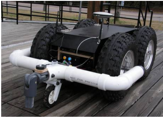
Figure 2-2 RMP 400- Note: Tow Bar, encoder, DGPS and 2 way communications
