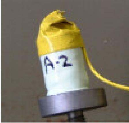
Composition pressed into 15 gram  $\frac{3}{4}$ " diameter pellets. Sides of pellets inhibited to burn linearly. Ignition slurry and electric match or firecracker fuse attached to top of pellet for performance testing.
