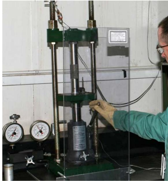
Figure 10. Laboratory Pellet Press and Flare Pellet Prepared for Radiometric Testing
