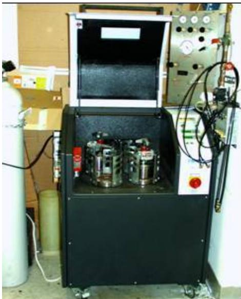
Figure 2. NJIT Scaled-up Planetary Mixer
