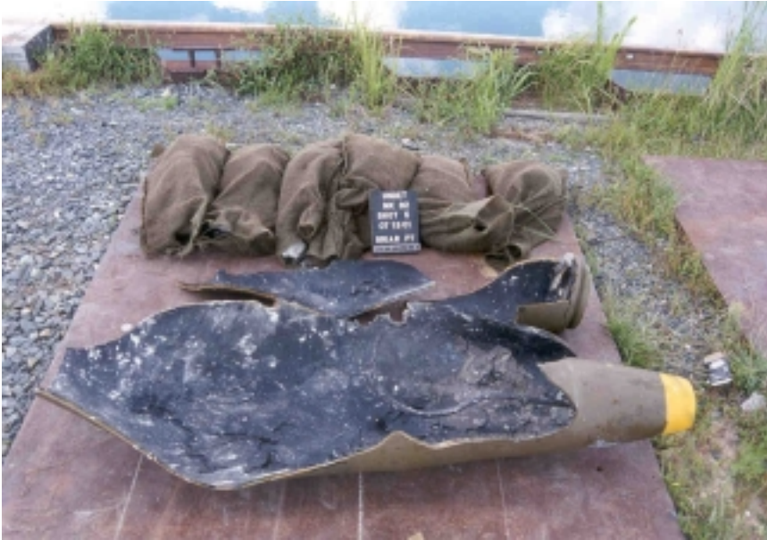
Figure 5. Typical Mk 82 Bomb Low-Order Test Result
