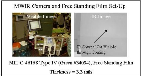
Figure E-24: IR Camera Cannot Detect IR Source through CARC Coating
