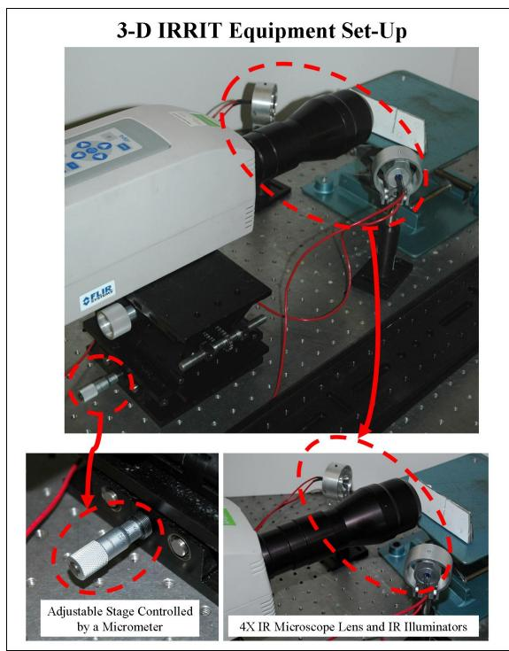
Figure E-35: 3-D IRRIT Equipment Set-Up
