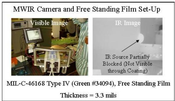
Figure E-25: IR Camera Cannot Detect IR Source through CARC Coating
