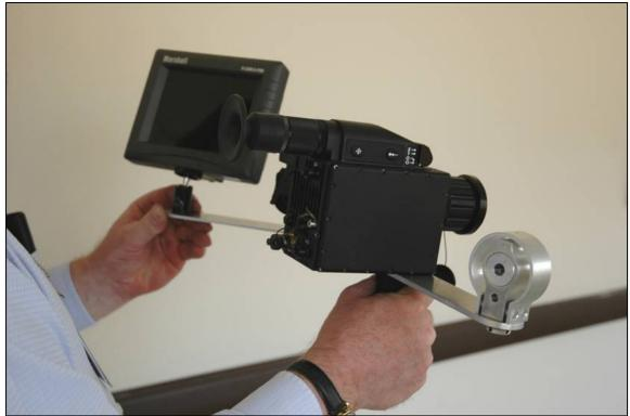
Figure E-15: FLIR MilCam w/IR Illuminators and LCD
