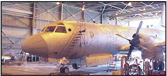
Figure 3-1: Paint Removed from P-3 Aircraft by Chemical Paint Stripping
