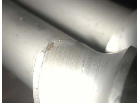
Figure 3-22. Example of Screw Damage on 40-mm TSE
