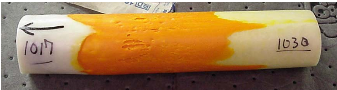
Figure 3-11. Inert Simulant Extruded Billet Showing No Flow Stagnation Points
