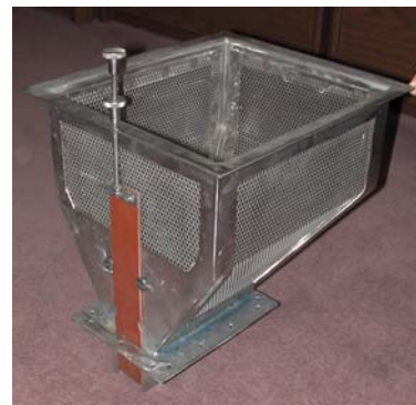
Figure 3-7. Engelhardt Vibratory Tray Feeder Installed (Left) and Vented Hopper (Right)
