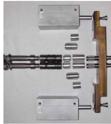
Figure 3-6. Die Lift-Off System (Left) and Barrel Screw Removal System Disassembled (Right)
