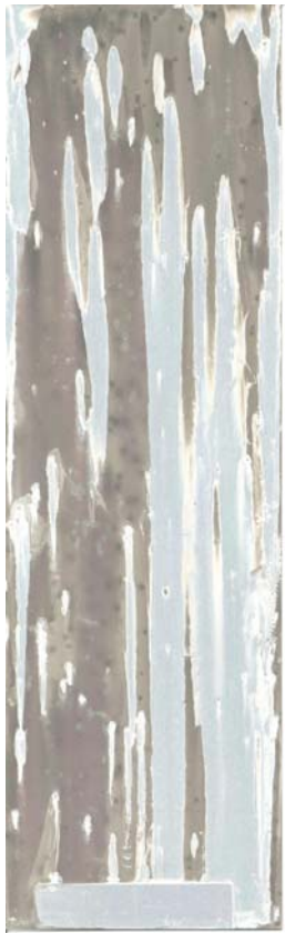
Figure 36: CFP seal for TFSA on AA2024 in comparison to chromate and DI water controls
