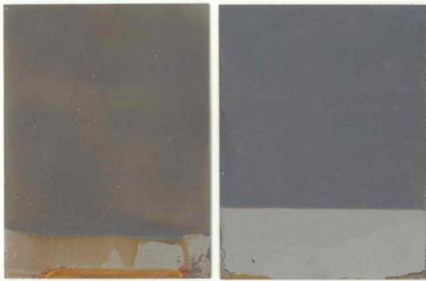
Figure 19: CFP on alumina-blasted 4130 steel – air-dried (left) and force-dried (right)
