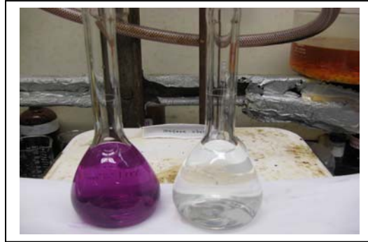
Figure 83: TCP and Alodine solutions exposed to sulfuric acid (left) and nitric acid (right) where the pink sample is the Alodine solution, while the clear solution is the TCP solution.
