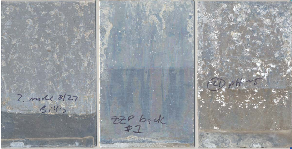
Figure 13: Corrosion protection of CFP-Sal (left), CFP-Z (center), and CFP (right) on AA2024-T3 after 48 hrs. ASTM B 117
