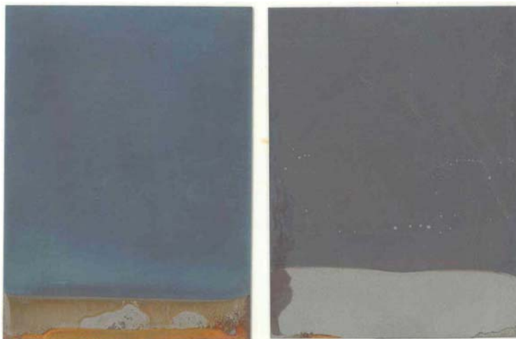
Figure 20: TCP on alumina-blasted 4130 steel – air-dried (left) and force-dried (right)
