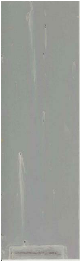
Figure 36: CFP seal for TFSA on AA2024 in comparison to chromate and DI water controls
