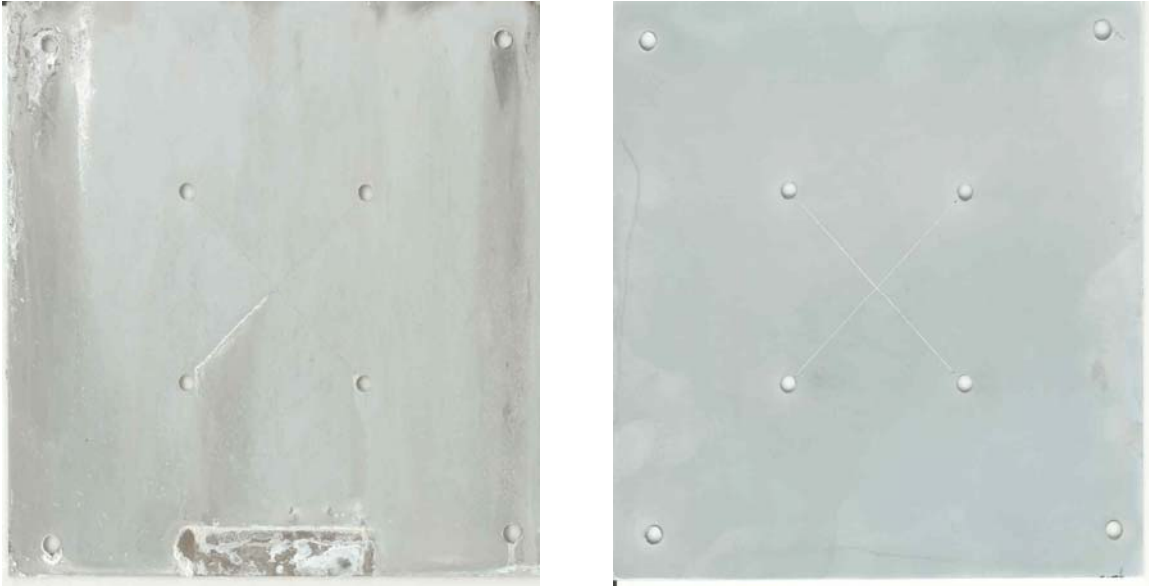
Figure 39: Alumiplate™ on 4130 steel – post-treated with CFP 6. After 4,200 hours ASTM B 117 (left) and as deposited (right)
