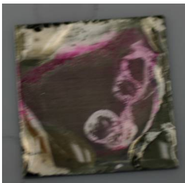
Figure 80: AA2024 after 16 hr in 1M sulfuric acid
