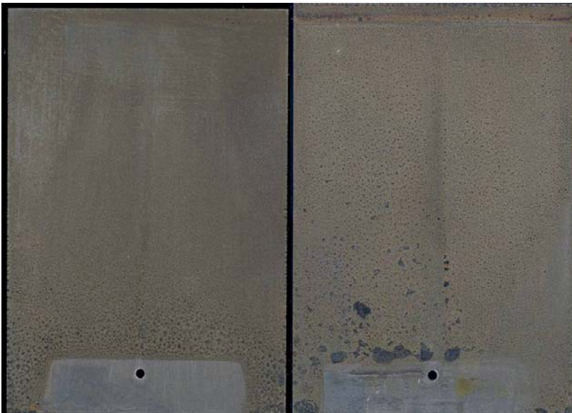
Figure 25: CFP on 4130 Steel after 1 Hour Humidity Testing – Best Processing Variation (#2 – left) and Worst Processing Variation ( #4 – right).
