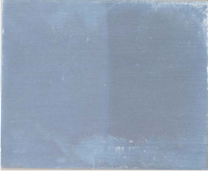
Figure 12: Improved corrosion protection of TCP-C AA2024-T3 panel after 500 hrs. ASTM B 117
