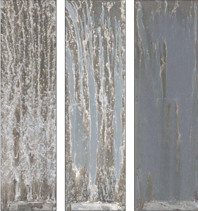
Figure 37: Poor corrosion resistance of PAA film with No Seal (left), TCP – 10 min. ambient (center), and TCP – 20 min. 100F (right) on AA2024-T3 after 72 hrs. ASTM B 117
