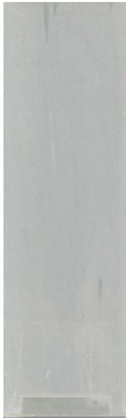
Figure 36: CFP seal for TFSA on AA2024 in comparison to chromate and DI water controls
