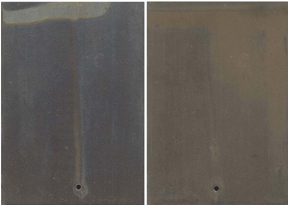
Figure 29: CFP on 4130 Steel after 4344 Hours Flash Rust Testing – Best Processing Variation (#3 – left) and Worst Processing Variation (#2 – right).
