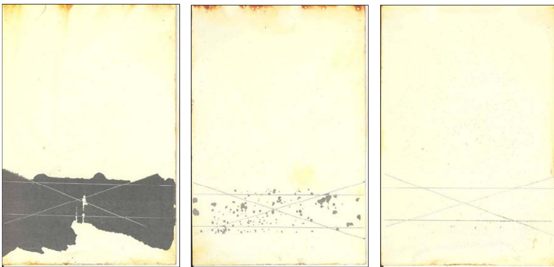
Figure 24: 7-day WTA testing of Acetone-Wipe (left), Grit-Blast (center), and Grit-Blast/TCP (right) on 4340 with MIL-DTL-53022 Type I
