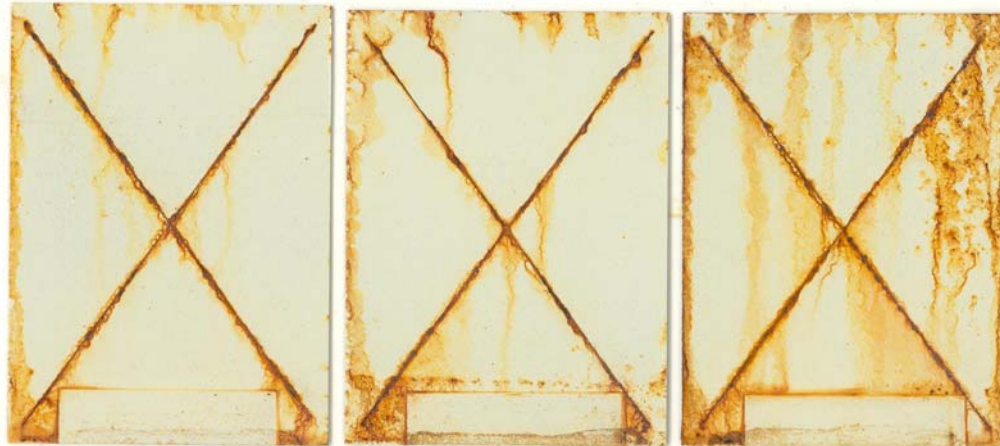
Figure 22: Grit-blasted 4130 steel with CFP/MIL-P-53022 – 168 hrs. B 117
