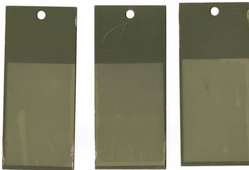
Figure 92: One component near zero VOC coating after 800 hours QUV exposure
