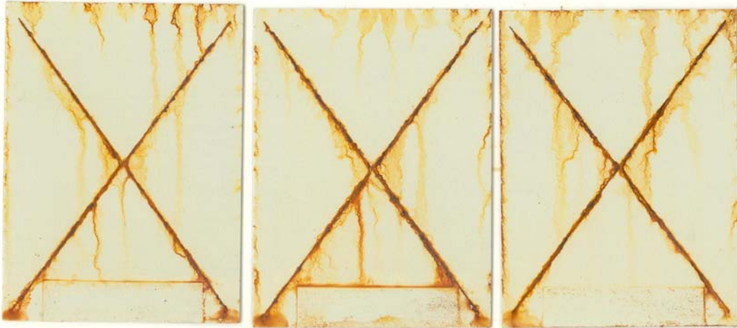
Figure 21: Grit-blasted 4130 steel with TCP/MIL-P-53022 – 168 hrs. B 117
