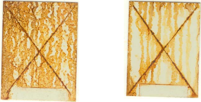
Figure 23: Grit-blasted (left) and acetone-wiped (right) 4130 steel control with MIL-P-53022 – 168 hrs. B 117
