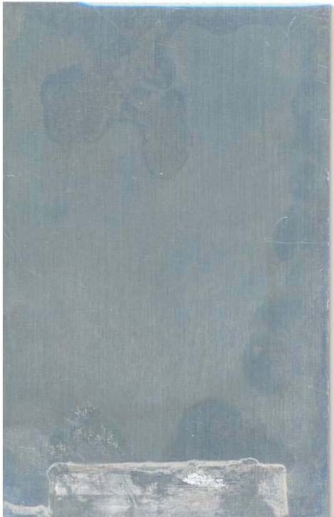
Figure 14: Improved corrosion protection of CFP-Z on AA6061-T6 after 672 hrs. ASTM B 117
