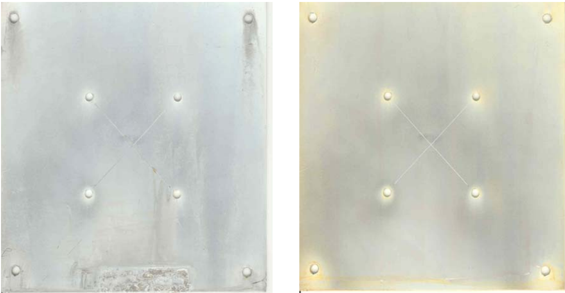
Figure 40: Alumiplate™ on 4130 steel – post-treated with Alodine™ 1200S. After 4,200 hours ASTM B 117 (left) and as deposited (right)
