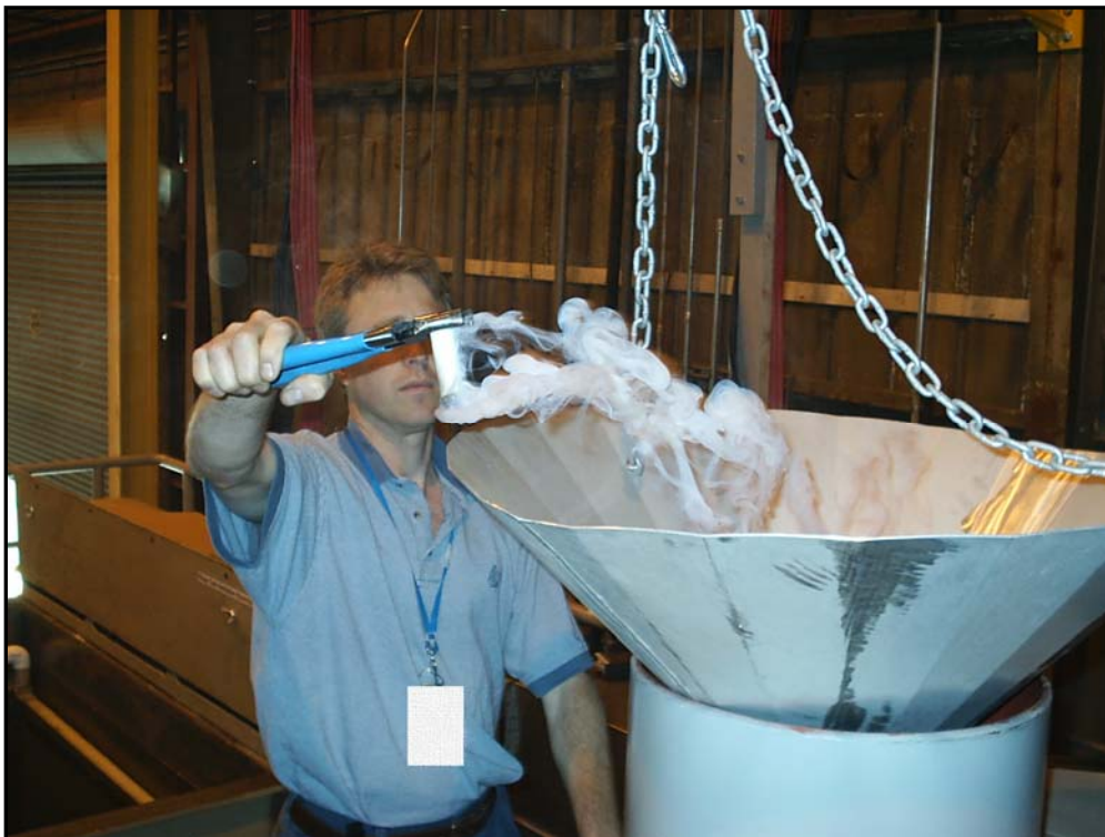
Figure 2-14. Ventilation Smoke Test with Chemical Add Funnel Inserted in Ventilation Plenum
