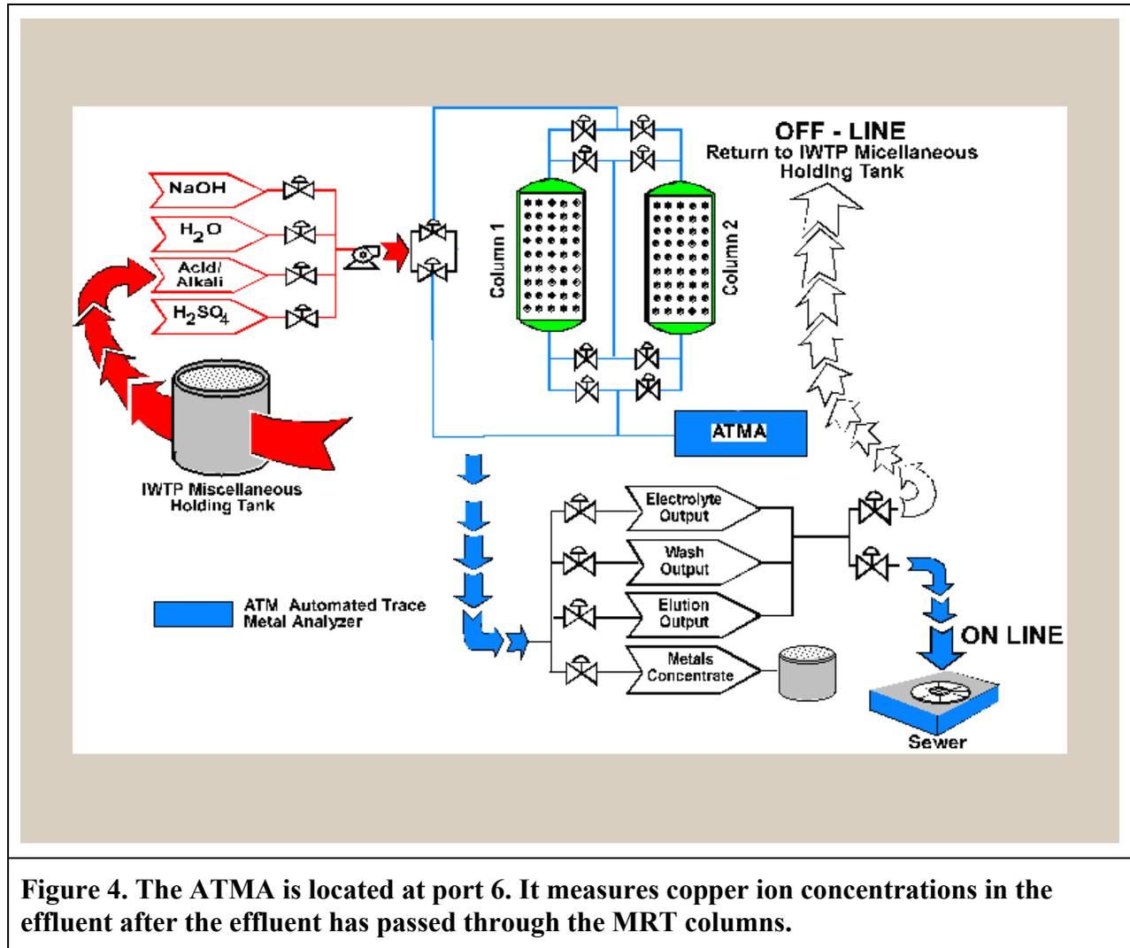
**Figure 4. The ATMA is located at port 6. It measures copper ion concentrations in the effluent after the effluent has passed through the MRT columns.**
