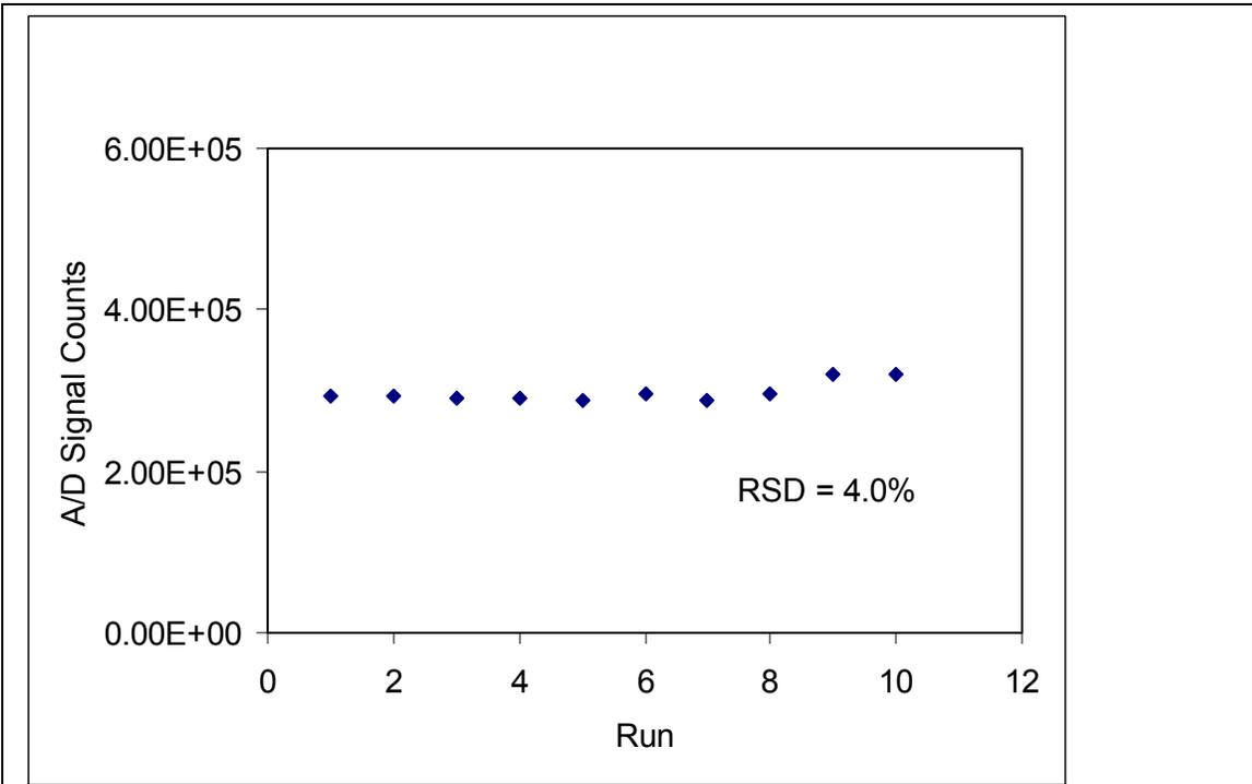
**Figure 19. A single water sample was spiked with selenium(IV) to 32 μg/l and measured 10 times. The relative standard deviation for this set is 4.0%.**
