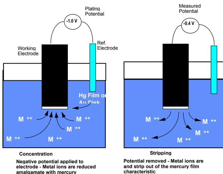
**Figure 2. Potentiometric Stripping of Trace Metals is a two step process consisting of a concentration step where the metal ions are amalgamated on the electrode and a stripping step where the metals are removed.**
