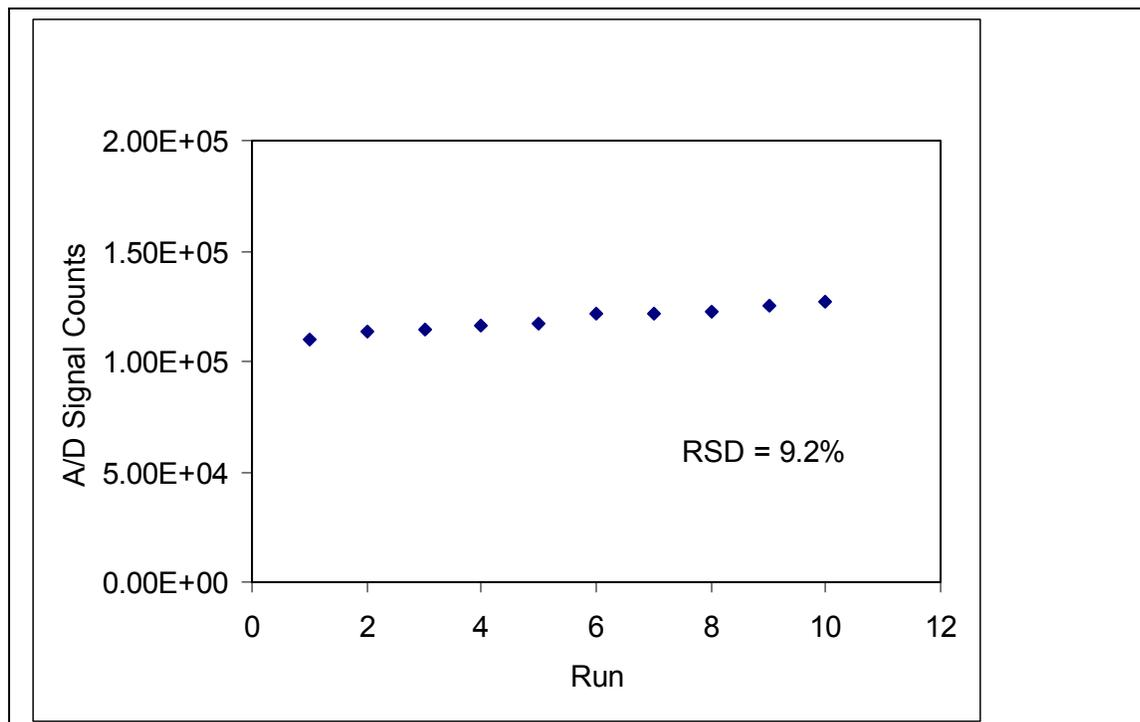
**Figure 16. A single water sample was spiked with mercury(II) to 32 µg/l and measured 10 times. The relative standard deviation for this set is 9.2%32ppb**
