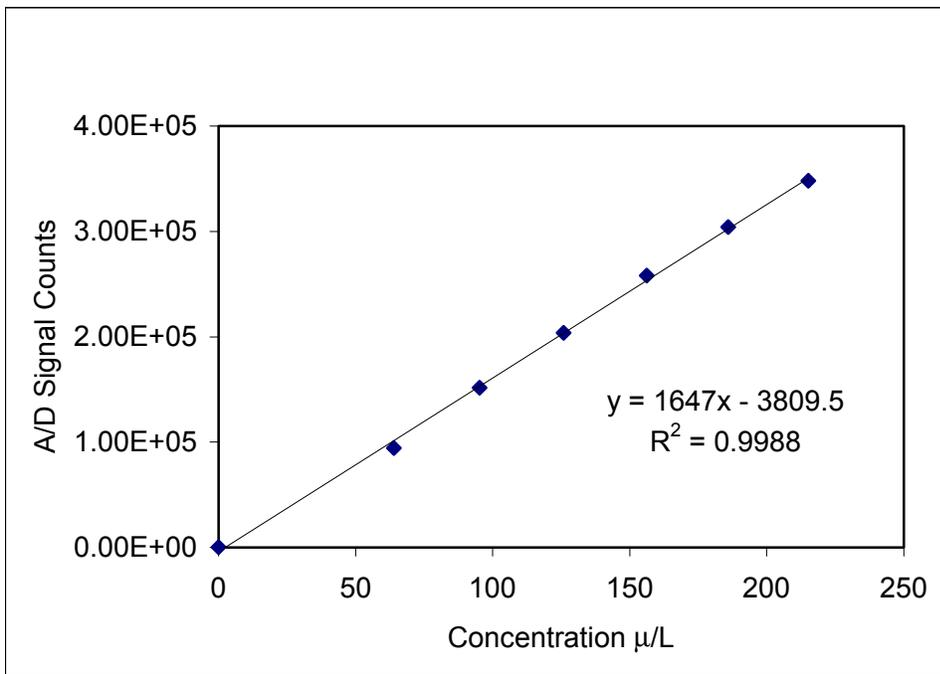
**Figure 12. Response of the ATMA to water samples spiked with 64-215μg/l copper(II).**
