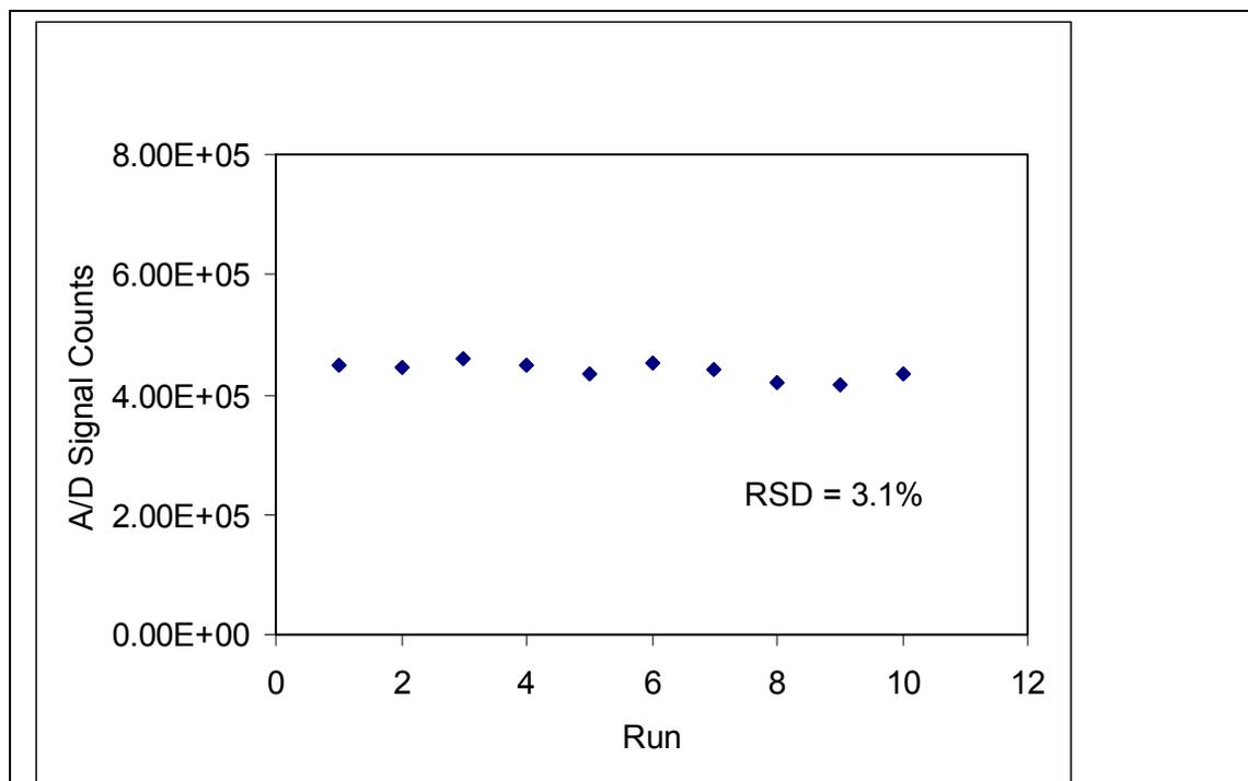
**Figure 10. A single water sample was spiked with chromium(VI) to 16 µg/l and measured 10 times. The relative standard deviation for this data set is 3.1%.**
