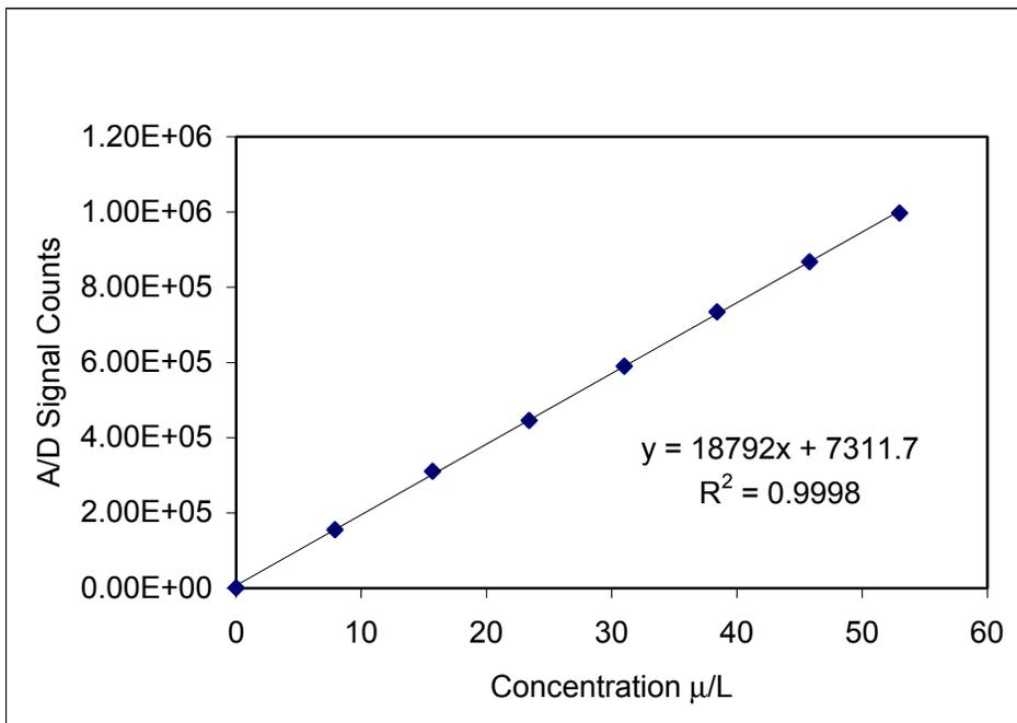
**Figure 5. Response of the ATMA to water samples spiked wit 0-53 $\mu$ g/l Arsenic(III)**
