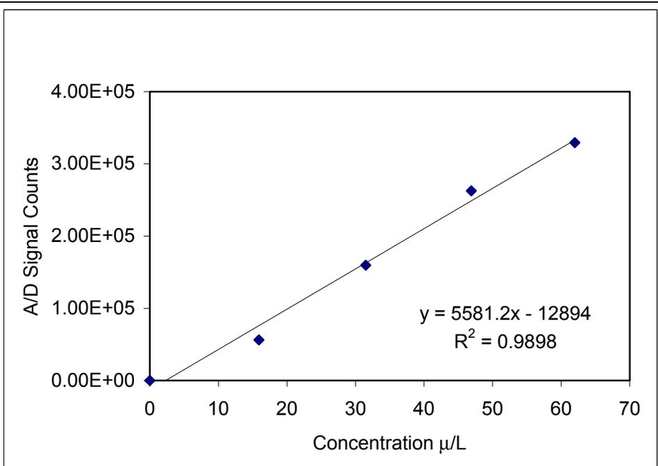
**Figure 9. Response of the ATMA to water samples spiked with 15-65 µg/l chromium(VI).**
