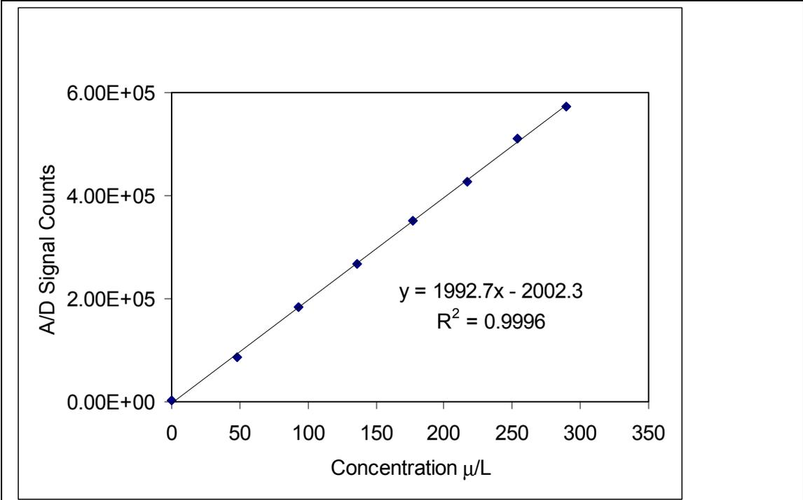
**Figure 18. Response of the ATMA to water samples spiked with 48-288μg/l selenium(IV).**
