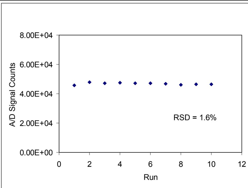
**Figure 13. A single water sample was spiked with copper(II) to 32 μg/l and measured 10 times. The relative standard deviation for this set is 1.6%**
