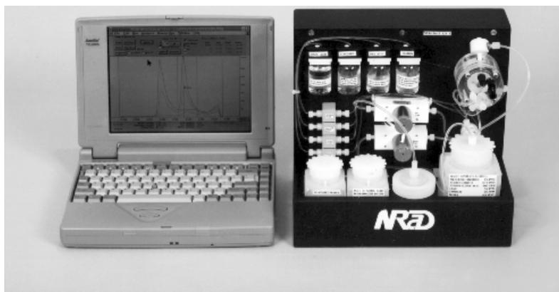
**Figure 1. The Trace Metals Analyzer is composed of a computer and electronic boards (on the left and a wet chemistry section (on the right).**
