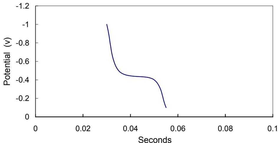
**Figure 3. A potentiometric Stripping Curve. While a metal is oxidizing and stripping off of the electrode the potential remains constant. The width of this plateau is proportional to the original concentration of metal ion in solution.**
