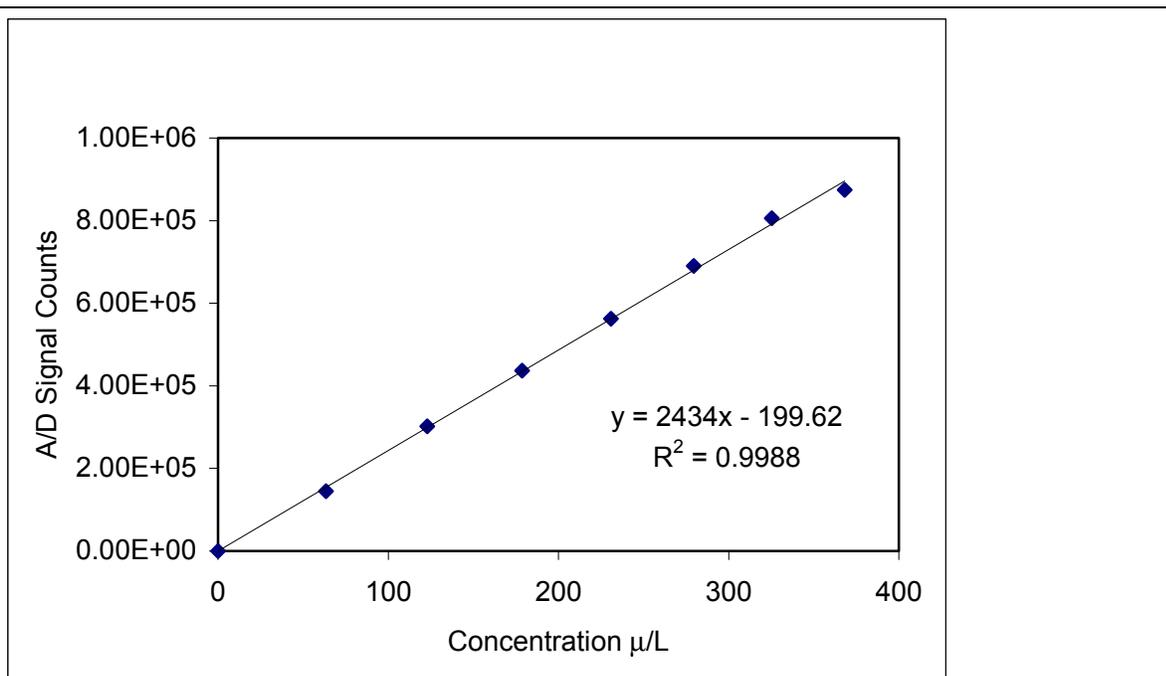
**Figure 6. Response of the ATMA to water samples spiked wit 63-368 $\mu$ g/l Arsenic(III)**
