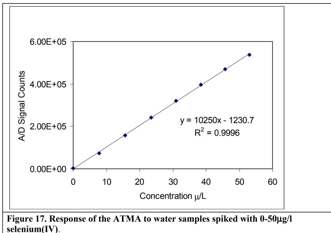
**Figure 17. Response of the ATMA to water samples spiked with 0-50µg/l selenium(IV).**
