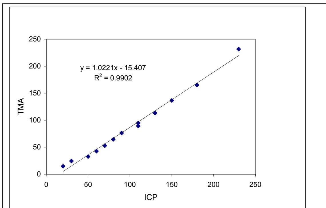
**Figure 20. Comparison of the ATMA copper measurements with grab samples measured using an ICP-MS (EPA Method xxx). The ATMA measurements in µg/l are on the Y axis and the ICP-MS grab sample measurements in µg/l are on the X axis. Measurement and sampling was done at Port 6 of the MRT. Grab samples were collected every 30 minutes. The MRT was run until the copper concentration reached 230µg/l.**
