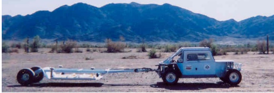
Fig. 2 – MTADS GEM array surveying at the YPG UXO Demonstration Test Site
