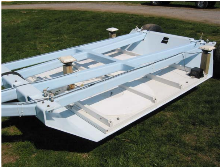
Fig. 1 – MTADS GEM-3 array shown mounted on the EMI sensor platform with three-member GPS array and IMU shown
