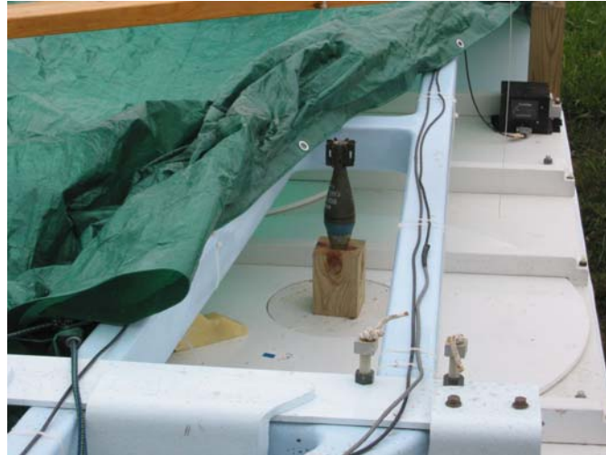
Figure 23 – Library response data being acquired for a 60-mm mortar
