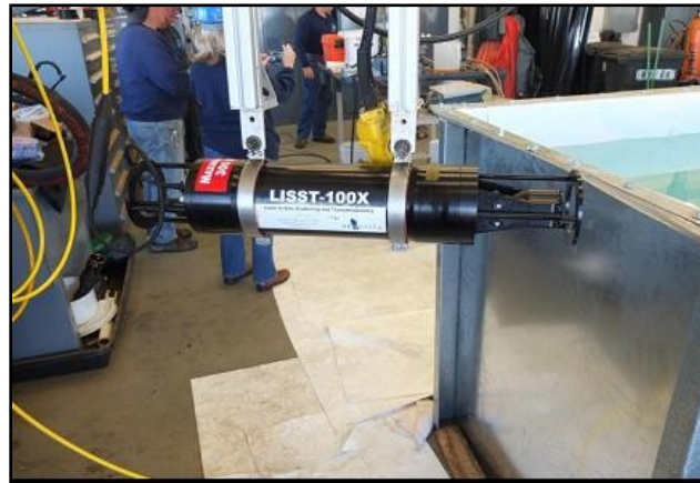
Figure A-5. LISST suspended from hoist.
