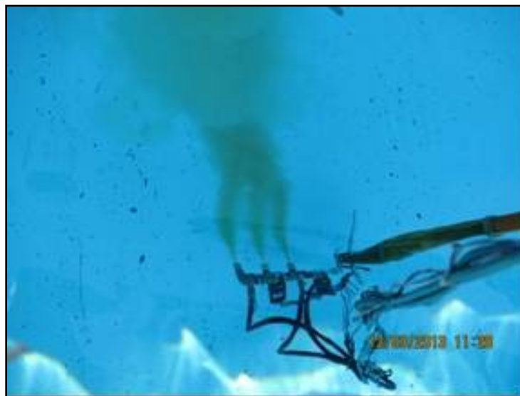
Figure 4. Creating an oil plume in the large tank.
