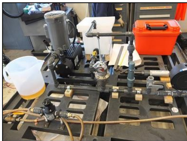
Figure A-2. Oil delivery pump system.
