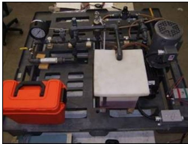
Figure 3. Oil dispensing system.
