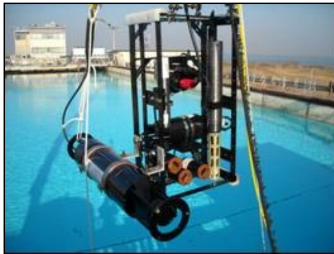
Figure 19. LISST attached to WINDOW sensor cage.
