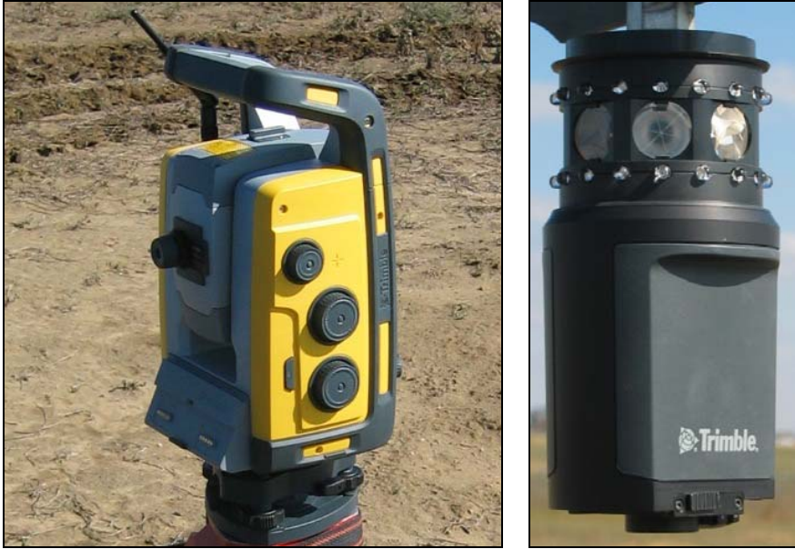
Figure 4. The new Trimble SPS930 (left) uses radio modems to send commands and position data to and from a portable controller while tracking an active prism (right) that has an IR glow from the ring of LEDs above and below the ring of mirrors.
