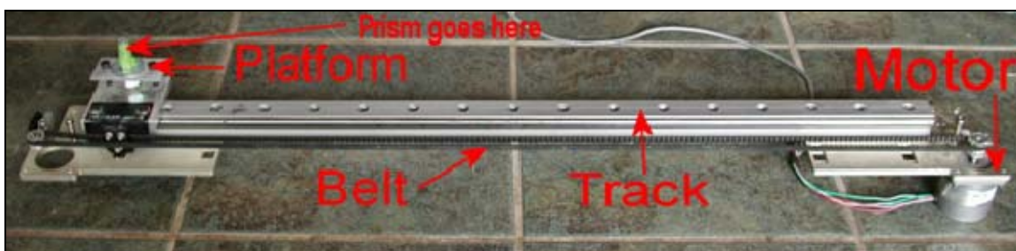
Figure 22. The stepper motor moves the test platform down the 0.83 m track in 11.8 seconds. The prism attaches to the platform while the DAS collects two platform position data streams from the microcontroller and the gun.
