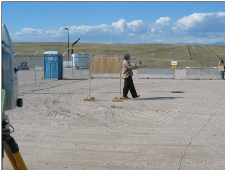
Figure 59. The RTS unit regains lock on the prism.
