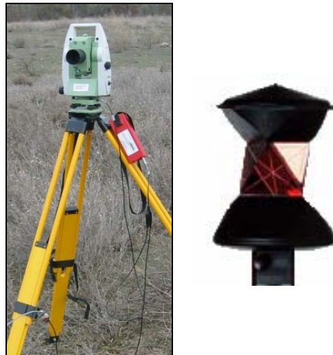
Figure 1. Leica TPS 1203 and 360° passive prism.
