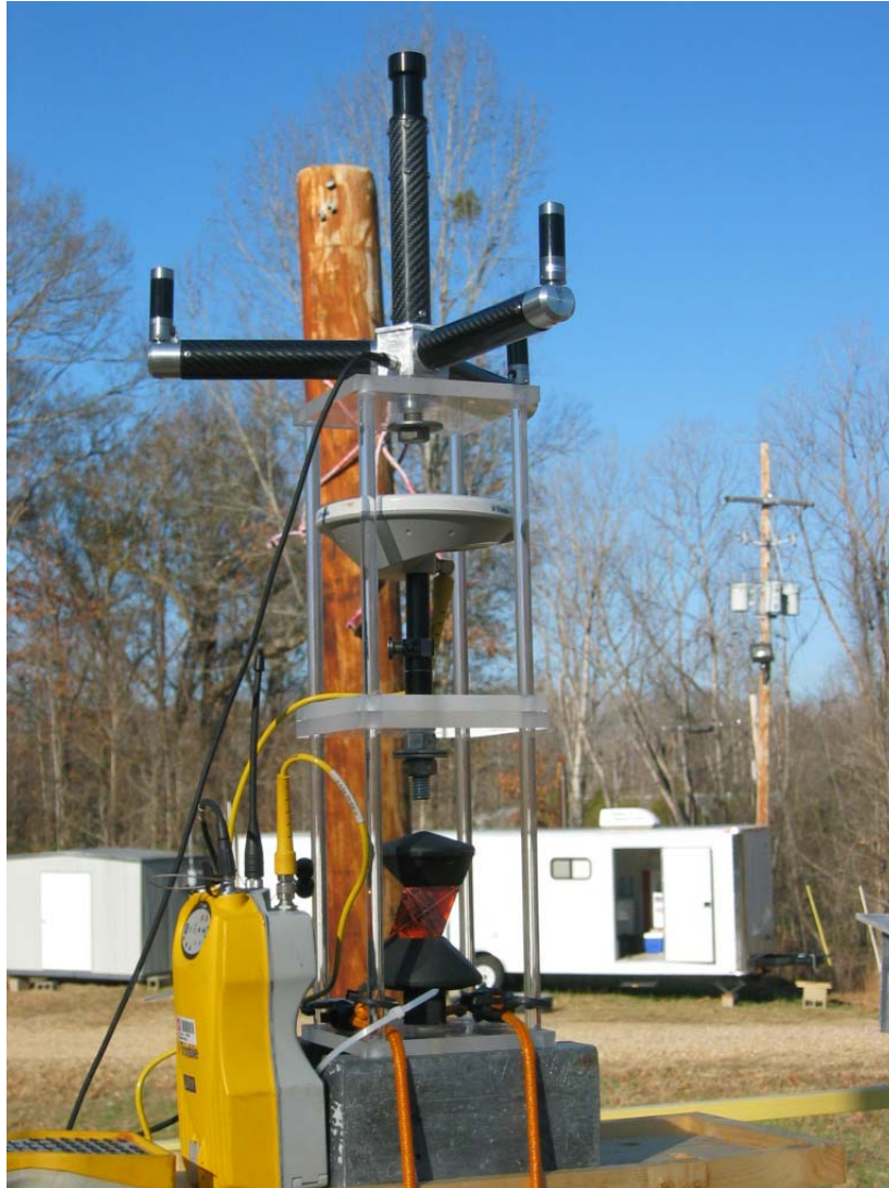
Figure 14. The tiered mount held the ArcSecond detector (top), the GPS antenna (middle) and Leica prism (bottom) securely to the trolley of the test stand.
