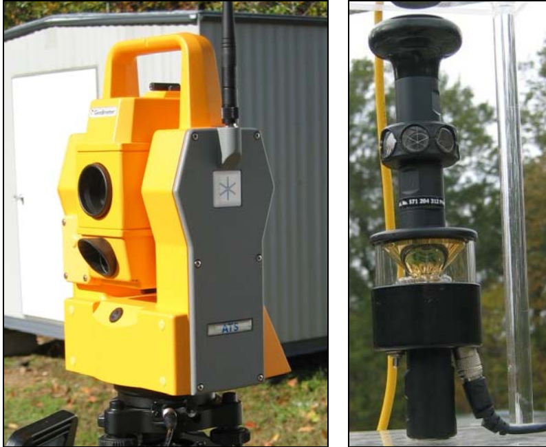
Figure 3. The Trimble ATS600 (left) searches and tracks the IR glow from the ring of LED lights on the active prism (right).
