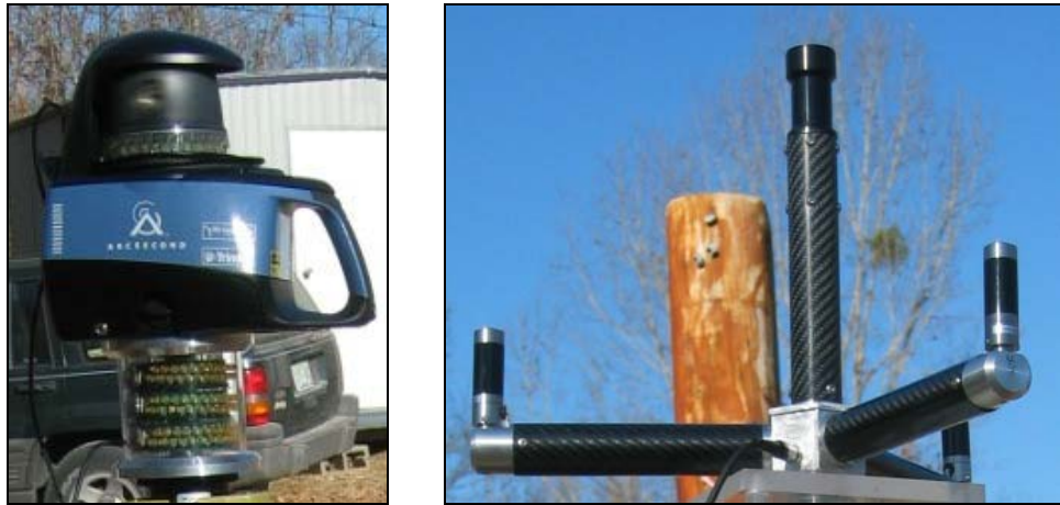
Figure 2. ArcSecond gun with rotating laser and flashing LED array (left) and the laser light detector which acts as the prism (right).
