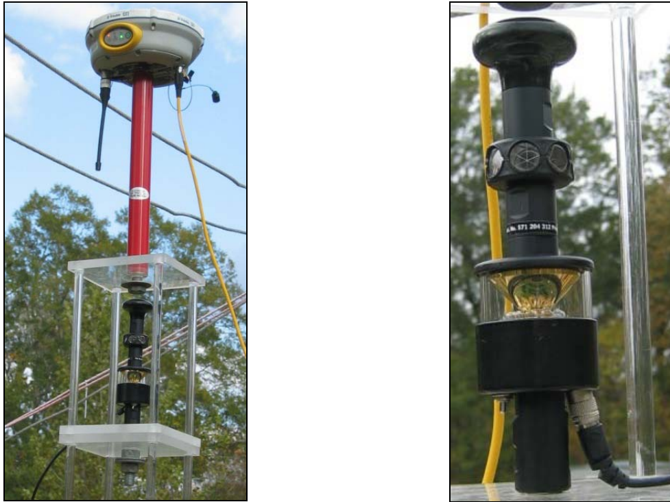
Figure 16. 3-Tiered Plexiglas mounting platform (left) and up close photo of the active prism (right). Below the reflective glass prism is a ring of LEDs that pulsate making this an active prism.
