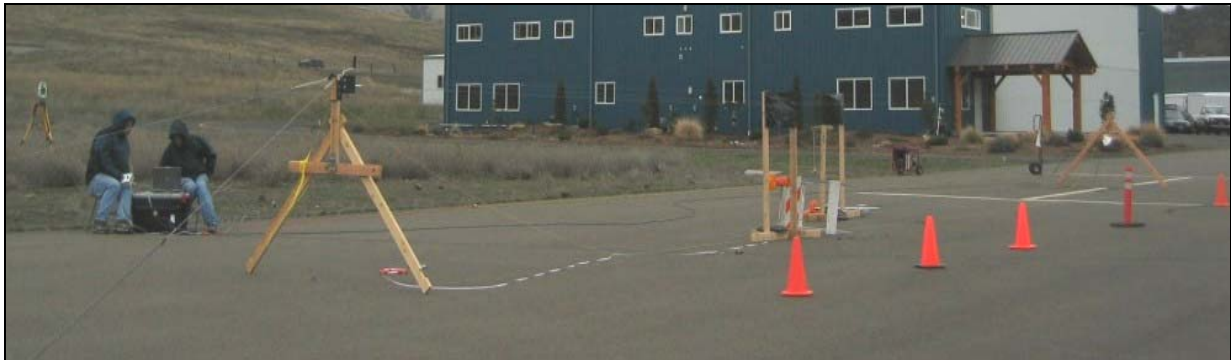
Figure 61. Equipment layout for the LOS tests conducted for performance assessment of the multi-gun positioning technology.
