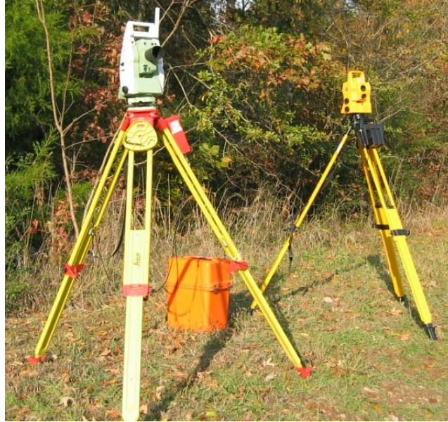
Figure 15. Leica TPS1203 (left) and Trimble ATS (right) stationed to the northwest of the ERDC Test Stand for laser assessment tests.
