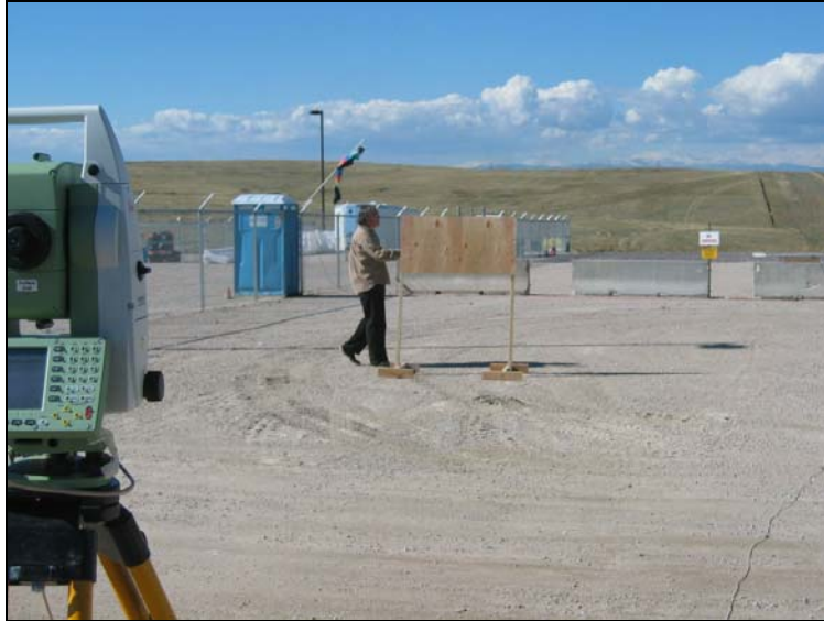
Figure 58. The prism is blocked by the plywood obstruction.
