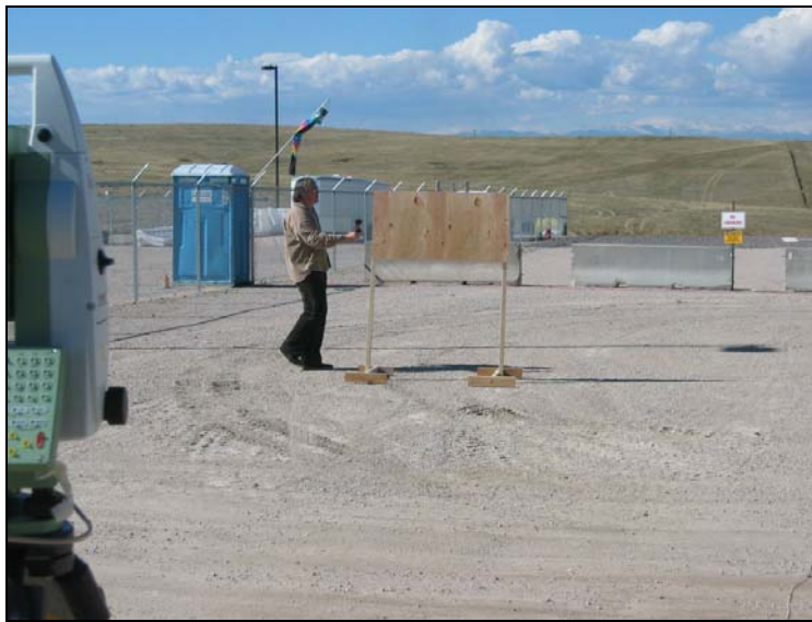
Figure 57. The RTS unit tracks the prism unit obscured by an obstruction.
