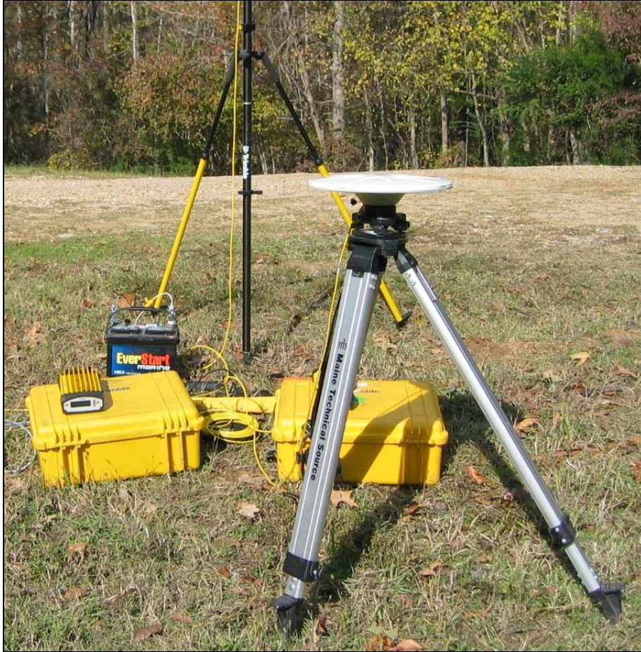
Figure 5. Base-station setup used to provide corrections to a rover that operates in RTK mode.
