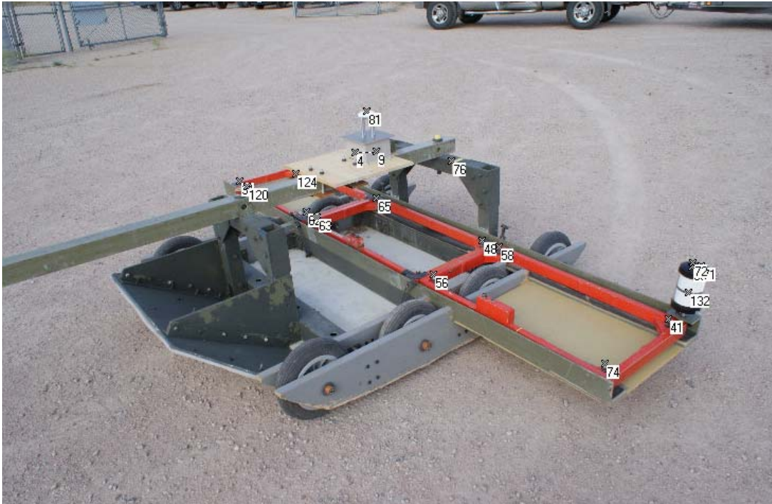
Figure 14: Sky Research EM61 towed array with GPS receiver (point 81), HG1700 IMU (points 4 and 9) and MT900 prism (point 132). The numbers delineate reference points used to define the precise geometry of the array through analysis of multiple photographs taken from different positions.
