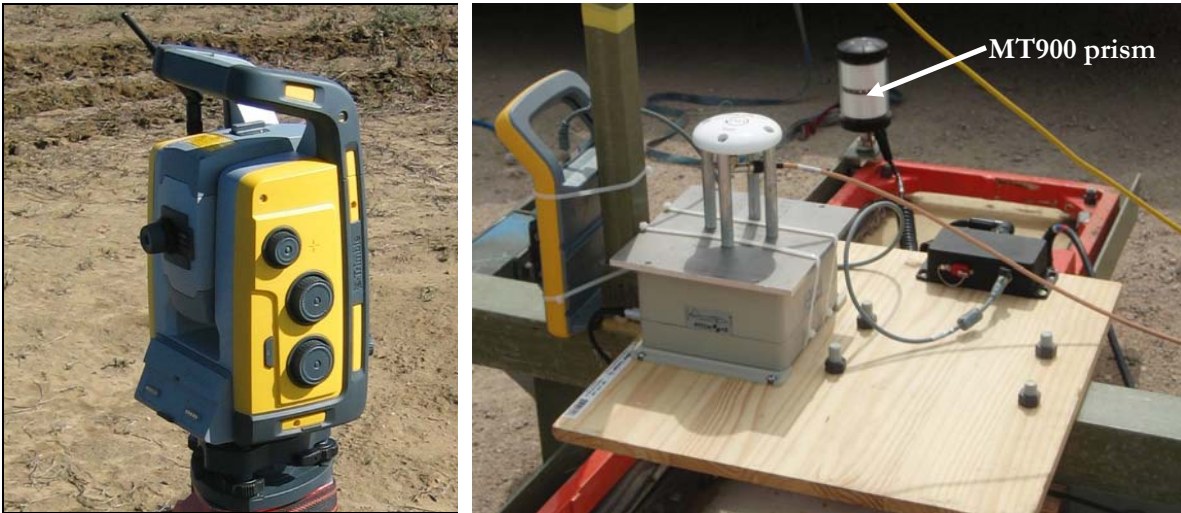
Figure 15: The new Trimble SPS930 (left) uses radio modems to send commands and positions data to and from a portable controller while tracking the prism on the bottom corner of the towed array.
