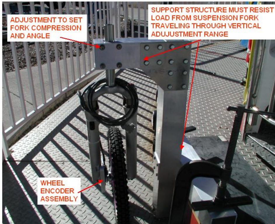
Figure 6: Bicycle wheel assembly mounted to carousel.
