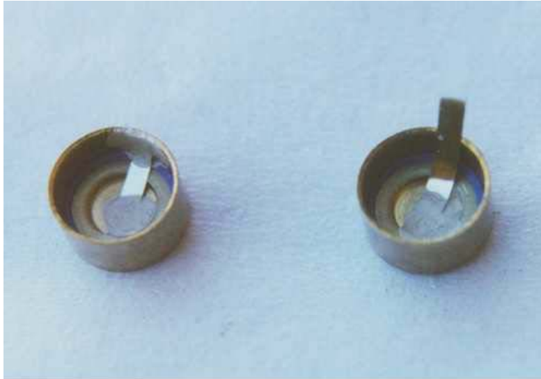
Figure 2 – Exploding Foil Primer Configuration
