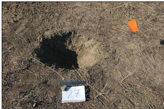
Figure 4. Example of a calibration site crater with a diameter of 0.75 m and depth of 0.4 m.
