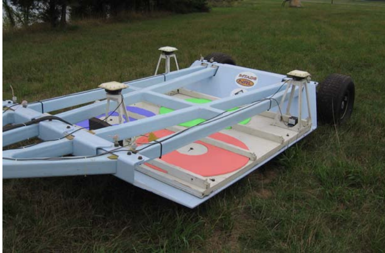
Figure 2-6 – MTADS GEM-3 array mounted on the EM sensor trailer. In addition to the three GEM sensors, note the three GPS antennae and the IMU for platform motion measurement.
