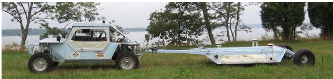
Figure 2-7 – MTADS GEM-3 array in operation pulled by the MTADS tow vehicle
