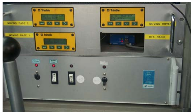
Figure 2-9 – GEM-3 array control electronics and GPS receivers
