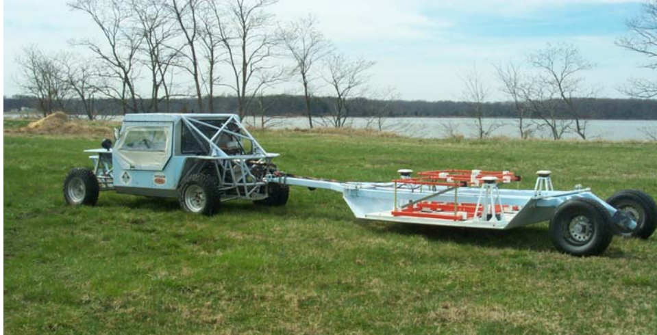
Figure 2-3 – MTADS EM61 MkII array pulled by the MTADS tow vehicle
