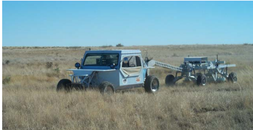
Figure 2-1 – MTADS tow vehicle and magnetometer array
