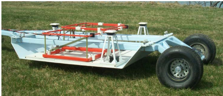
Figure 2-5 – Close-up of MTADS EM61 array with GPS and IMU
