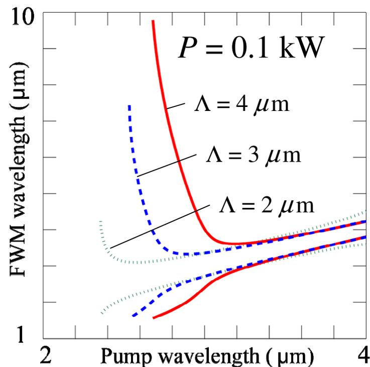
At  $P = 0.1 \text{ kW}$ ,  $\Lambda = 3 \mu\text{m}$  gives a large Stokes wavelength
