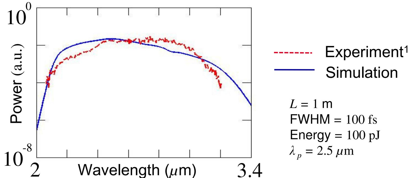
Measured nonlinear response can completely account for the supercontinuum generation
