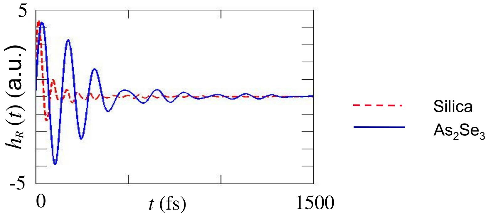
*Chalcogenide fiber has a longer response time than silica fiber*
