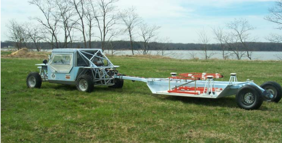
Figure 2-3 – MTADS EM61 array pulled by the MTADS tow vehicle
