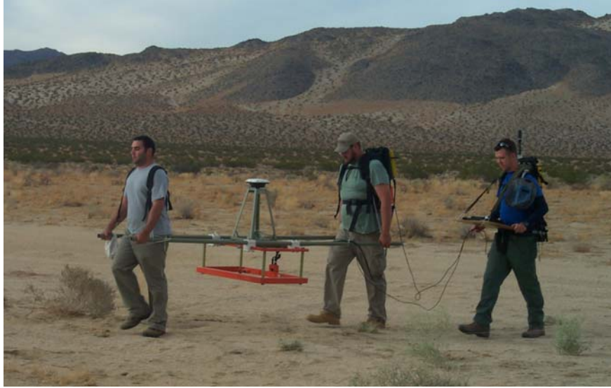
Figure 2-5 – Man-portable, litter-carried EM61 MkII sensor system
