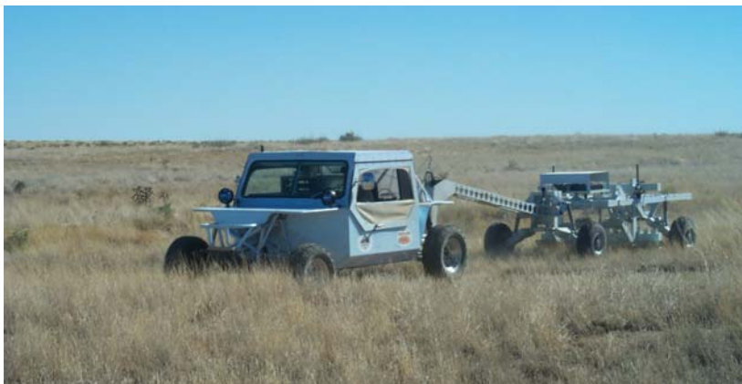
Figure 2-1 – MTADS vehicle towing the magnetometer array
