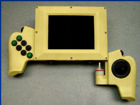
SSC-SD's Common OCU, which runs the Multi-Robot Operator Control Unit (MOCU)
