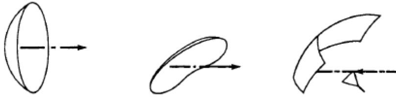
Figure 3. Common Reflective Antenna Shapes (from Skolnick 2008, 560)
