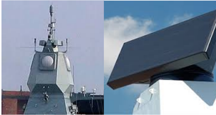
Figure 9. APAR (left) and SMART-L Radars (from Jane's 2013)
