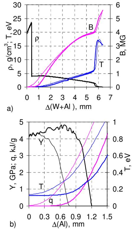
**Figure 3.** Simulated distributions of density  $\rho$ , magnetic field  $B$ , temperature  $T$ , Joule heating  $q$  and yield strength  $Y$  across the liner radius before liner/CMU impact in devices without ECS (heavy lines) and with ECS (11 and 15 in Table 1).  $\Delta = r - r_{in}$ ,  $r_{in}$  is inner radii of the liner's W layer (a) or Al layer (b).
