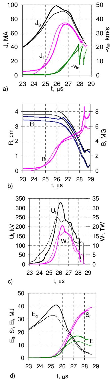
**Figure 4.** Simulated DEMG and load currents,  $I_g$  and  $I_i$ , velocity of inner liner surface  $v_{in}$ , radii of both liner surfaces ( $R_{in}$ ,  $R_{out}$ ) and magnetic field  $B_{out}$  on outer liner surfaces (a, b); FOS voltage  $U_f$ , power  $W_f$  and electromagnetic energy flux  $S_f$  delivered through FOS to the load, magnetic energies  $E_g$  and  $E_i$  in the DEMG and in the load (c, d), - in devices without ECS (heavy lines) and with ECS (11 and 15 in Table 1).
