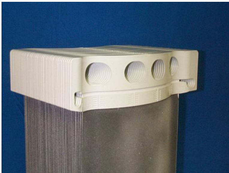
Figure 6. The upper end of a manufacturable low-flow conditioner.
