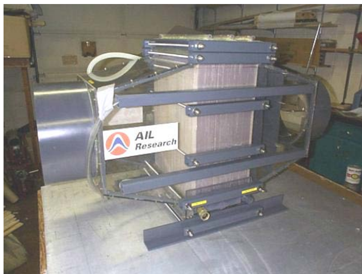
Figure 5. The first implementation of a low-flow conditioner.
