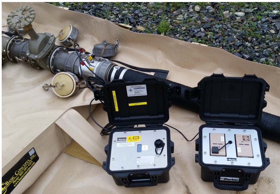
Figure 2. Parker icountOS light obscuration particle counter, BB-2590 battery box accessory, and fuel sampling port.
