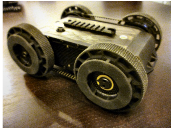
Figure 11. The Stingray with micro-knobby paddle wheels.
