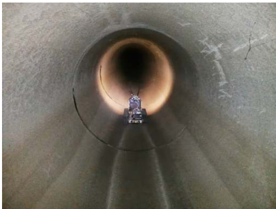
Figure 11: NREC MultiSense-SL mounted on iRobot PackBot mapping and localizing itself in storm drain
