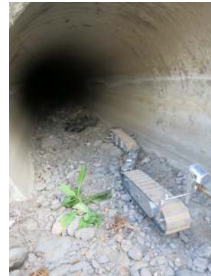
Figure 20: CTER platform in bend mode traversing rocky terrain in storm drain
