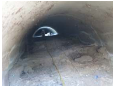
Figure 19: CTER platform traversing sandy stepped terrain in storm drain
