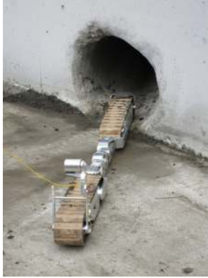
Figure 15: CTER platform about to enter a 45-cm storm drain
