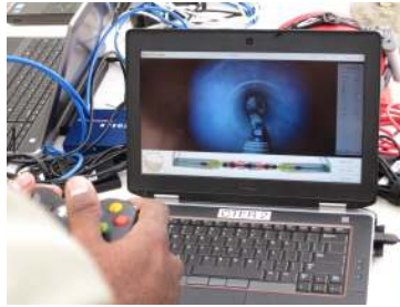
Figure 16: The video feed from the CTER platform as it traversed through the 45-cm storm drain
