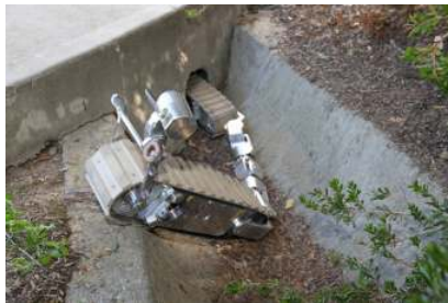
Figure 2: CTER platform fitting through tight passages
