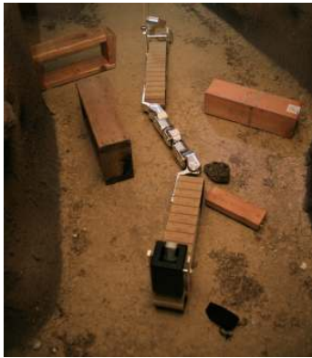
Figure 1: CTER platform maneuvering around obstacles in a narrow tunnel
