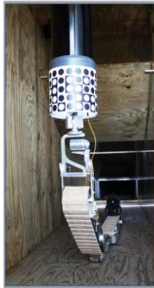
Figure 8: Deployment of the CTER platform through the borehole apparatus with attached localization fiducial
