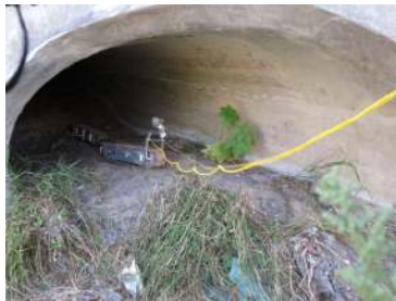
Figure 18: CTER platform traversing sandy terrain in storm drain
