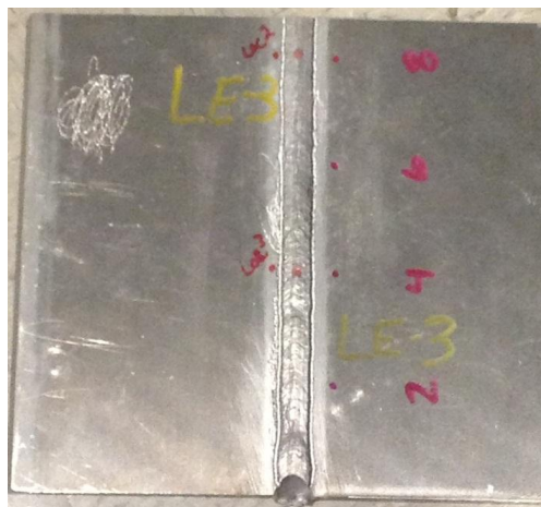
Figure 24. Two plates of non-sensitized, GMAW butt welded AA5456-H116. UIT is present at the toe of the weld and in a patch near the top left corner.
