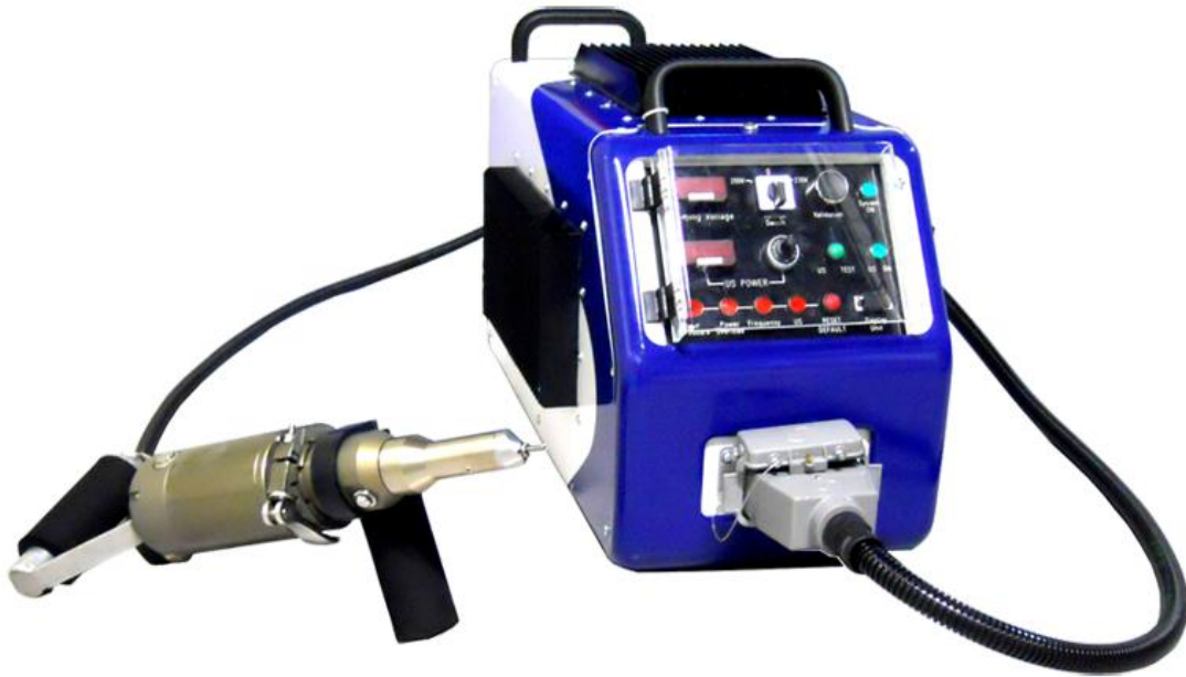
Figure 11. Sonats portable ultrasonic impact treatment machine (from [52]).
