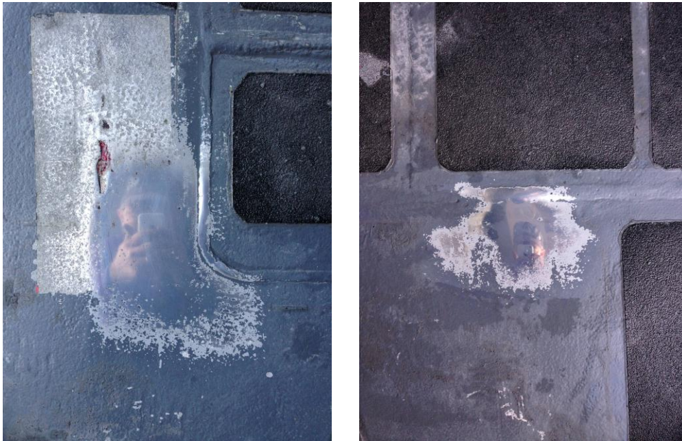
Figure 30. Shipboard sample location for residual stress measurements of field AA5456-H116. Sample position one is on the left (located at the rear corner of the air handler) and sample position two is on the right (located roughly at the midpoint of the air handler).
