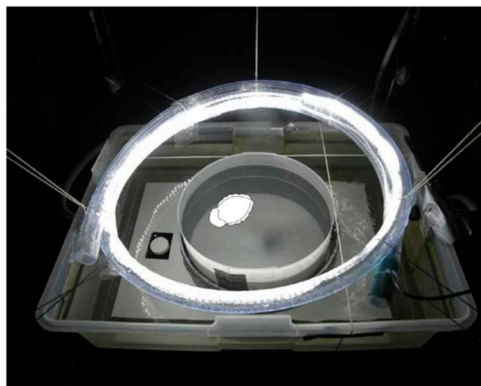
Figure 5.2 Experimental and photographic setup. The circular cuttlefish arena was placed in a rectangular tank supplied with seawater circulation. The setup was illuminated with a ring-shaped LED light, above which the camera was mounted looking down (not shown in photo). Black and white calibration targets were placed inside the rectangular tank (shown here on the left), out of the field of view of the animal in the circular arena and remained in the same location throughout the duration of the study.
