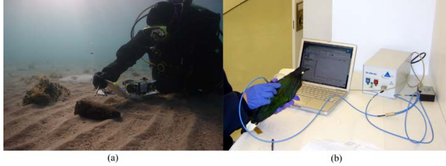
Figure 3.1 (a) A SCUBA diver extending the optical fiber attached to a spectrometer (in water and pressure proof housing) to record the spectrum of light reflected from the skin of a cuttlefish, in Urla, Turkey. Getting the optical fiber close enough to take accurate measurements from freely behaving animals in the wild is challenging. Photo credit: Derya Akkaynak. (b) Spectral measurements of a specimen can be recorded in a laboratory by getting the fiber as close to the specimen as possible without touching it. Photo courtesy of M.C. Stoddard & K. Zyskowski, taken at the Ornithology Collections of the Peabody Museum of Natural History, Yale University, New Haven CT.
