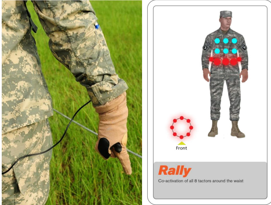
Figure 8. Hand gesture (left) and diagram of tactile vest activation pattern (right) for “rally.”
