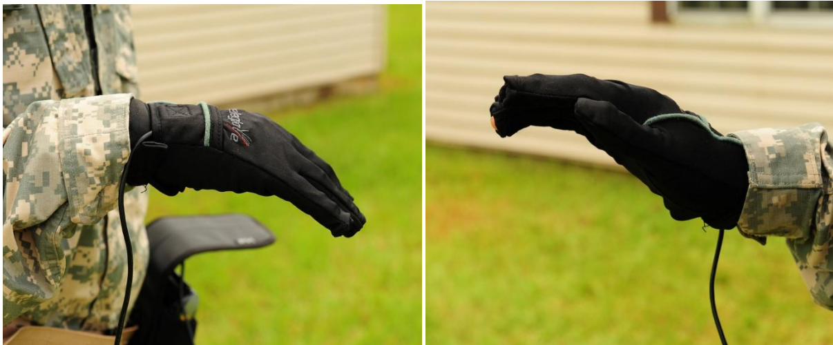
Figure 14. Forward robot control (left) and reverse robot control (right).
