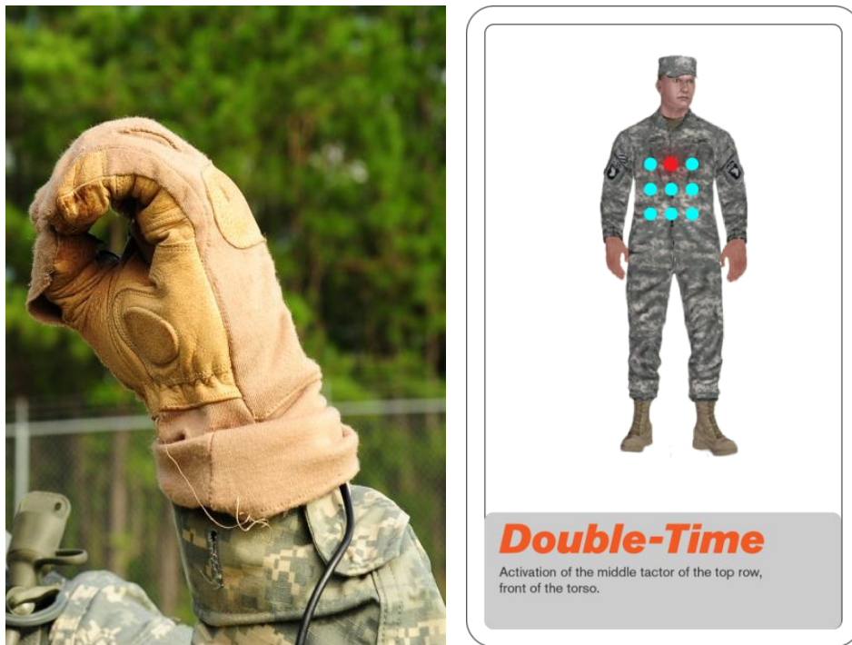
Figure 9. Hand gesture (left) and diagram of tactile vest activation pattern (right) for “double-time.”
