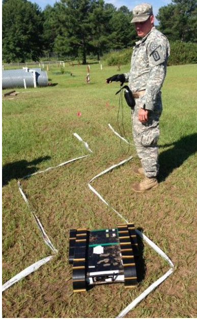
Figure 22. EOD specialist using instrumented glove to control robot maneuvers on the zigzag course.
