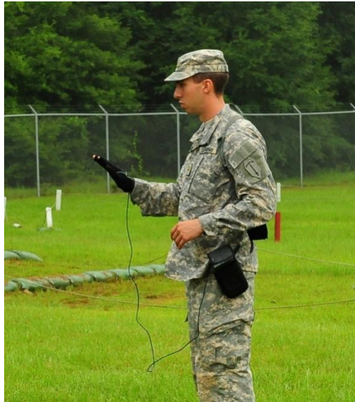
Figure 12. Soldier using instrumented glove for robot control.
