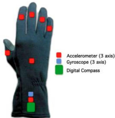
Figure 2. Instrumented ruggedized tactical glove used for Soldier communication.
