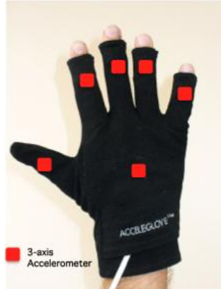
Figure 13. Acceleglove sensor placement diagram.
