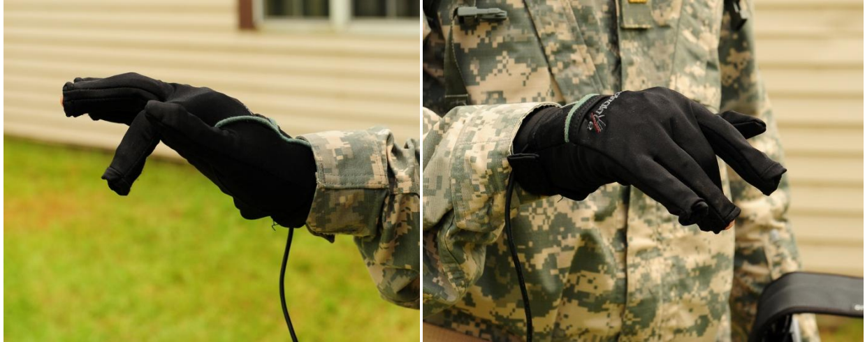
Figure 15. Left turn robot control (left) and right turn robot control (right).
