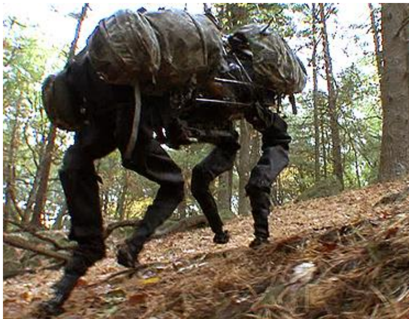
Figure 1. The LS3 BigDog in Action built by DARPA and Boston Dynamics (from Knowles, 2013)
