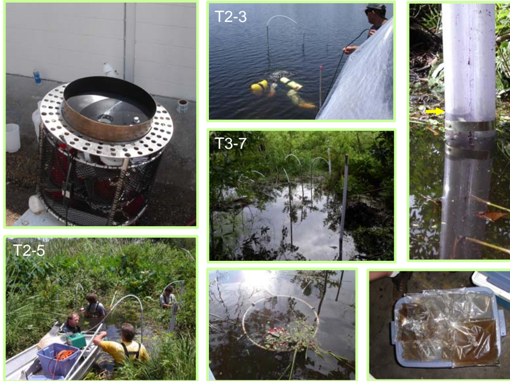
Figure 14. Field Deployment and Validation of the UltraSeep at Three Locations Along Druid Lake.
