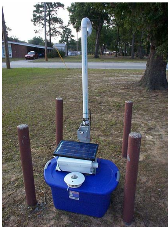
Figure 3 Picture of remote sensor and data logging system. An air-velocity transducer was mounted in 2-in outside diameter (OD) PVC piping attached to a groundwater monitoring well. A datalogger is located in the white box beneath the solar pane, and a 12V battery is contained in the blue tub.
