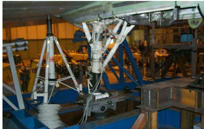
Figure 17. P3 Main Landing Gear Assembly with HVOF WC/17Co-Coated Components Mounted in Test Rig.
