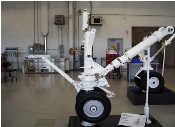
Figure 16. F/A-18 E/F Nose Landing Gear Assembly with HVOF WC/10Co4Cr-Coated Components Prior to Mounting in Test Rig at Messier-Dowty.
