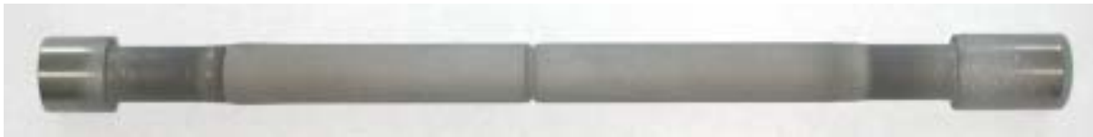
Figure 9. F-519, Type 1a.2 Specimen Coated with 0.010" WC/17Co.
