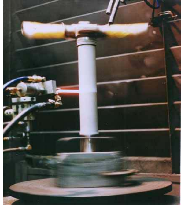
Figure 2. HVOF Spray of Landing Gear Inner Cylinder.
