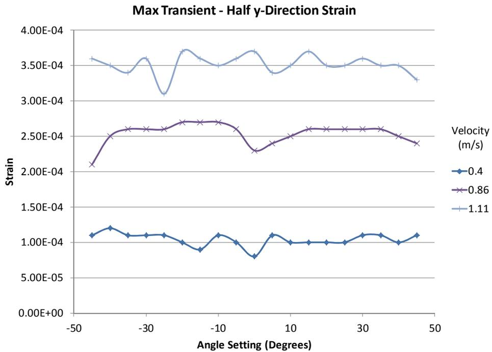
Figure 80 Framed composite maximum transient strain at half location in y direction for intermediate angles
