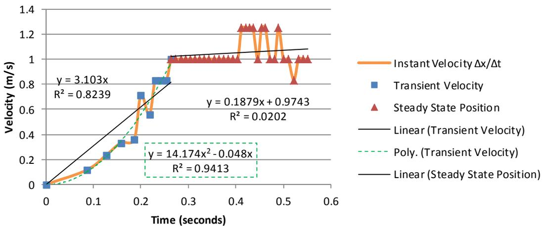
Figure 122 Frame velocity vs time at 7 Hz speed setting
