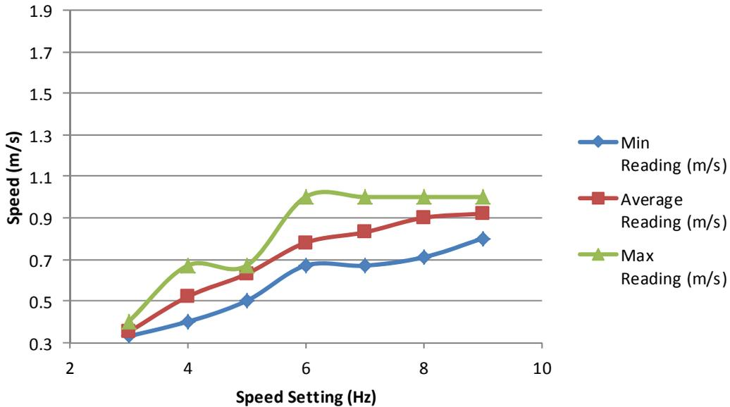
Figure 36 Frame starting steady state velocity in water
