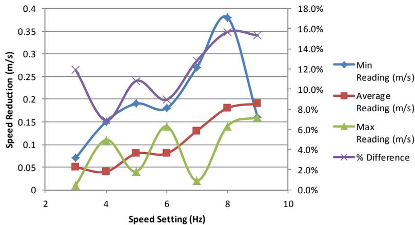
Figure 43 Change in speed from starting velocity to developed velocity in water
