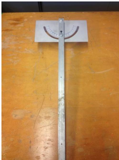
Figure 18 Angle selector with box tube test rig
