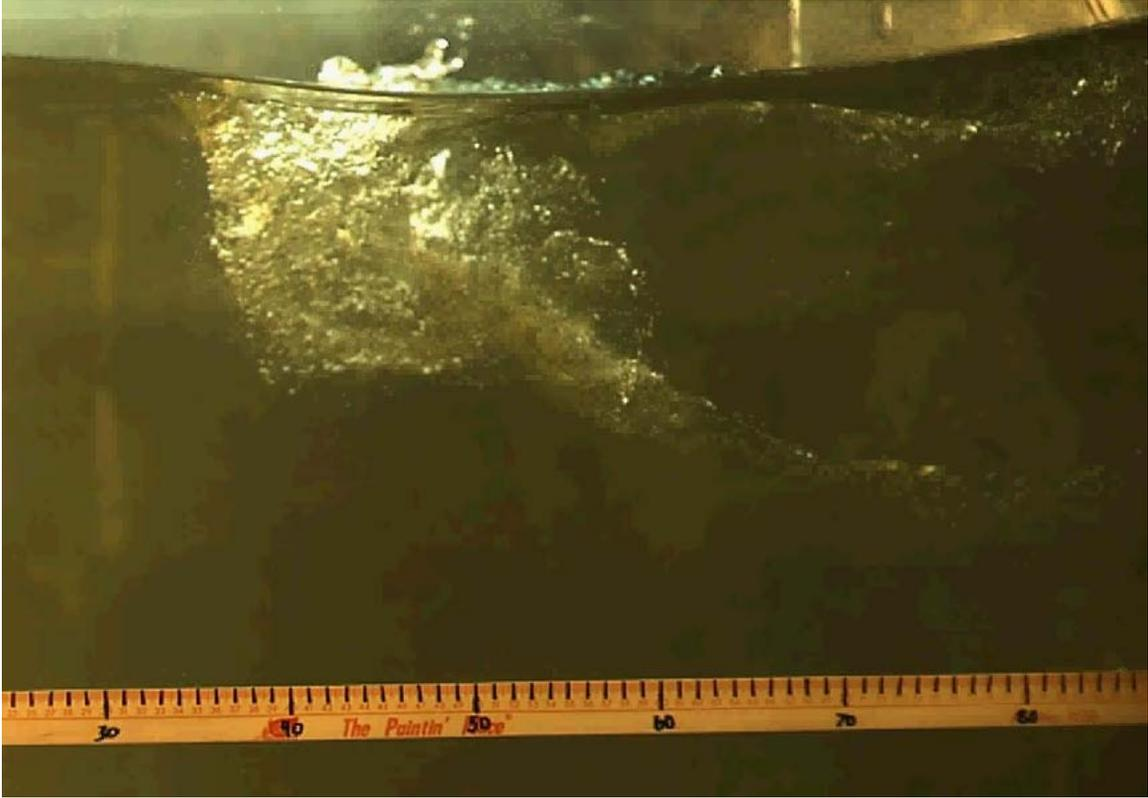
Figure 93 Bubbles from top of plate joining void behind plate for +30°
