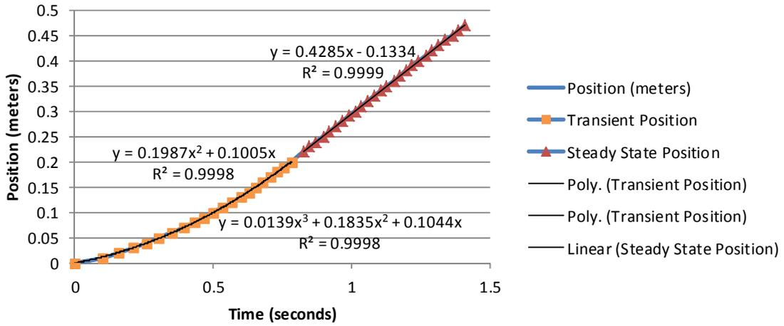
Figure 30 Frame position vs time at 3 Hz speed setting
