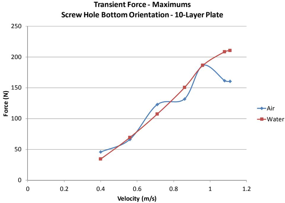
Figure 53 Maximum peak transient force for all speeds of 10-layer composite sample in bottom orientation
