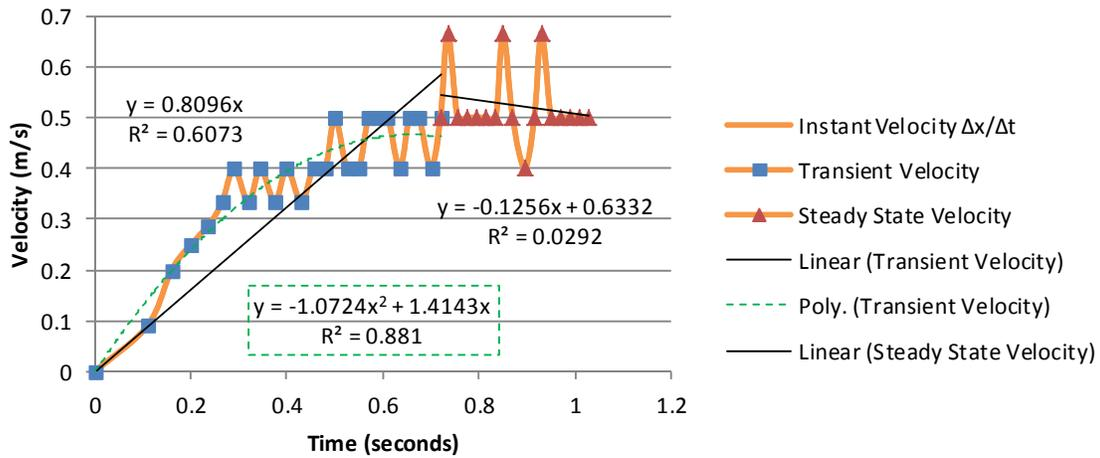
Figure 128 Frame velocity vs time at 4 Hz speed setting
