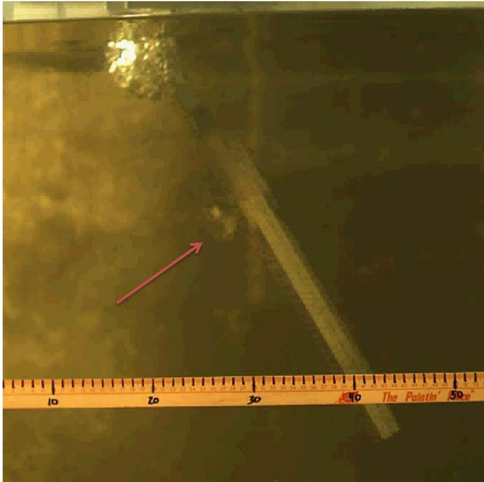
Figure 92 Development of bubbles from top of sample at  $+30^\circ$
