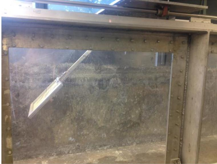
Figure 19 Angle selector mounted to carriage with frame attached to test rig at -45° in dry tow tank
