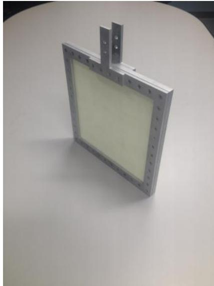
Figure 10 Angle view of frame test piece with six-layer composite
