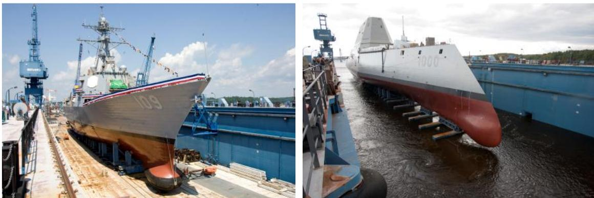
Figure 97 Comparison of DDG-51 to DDG-1000 waterline hull angles, from [20] and [21]
