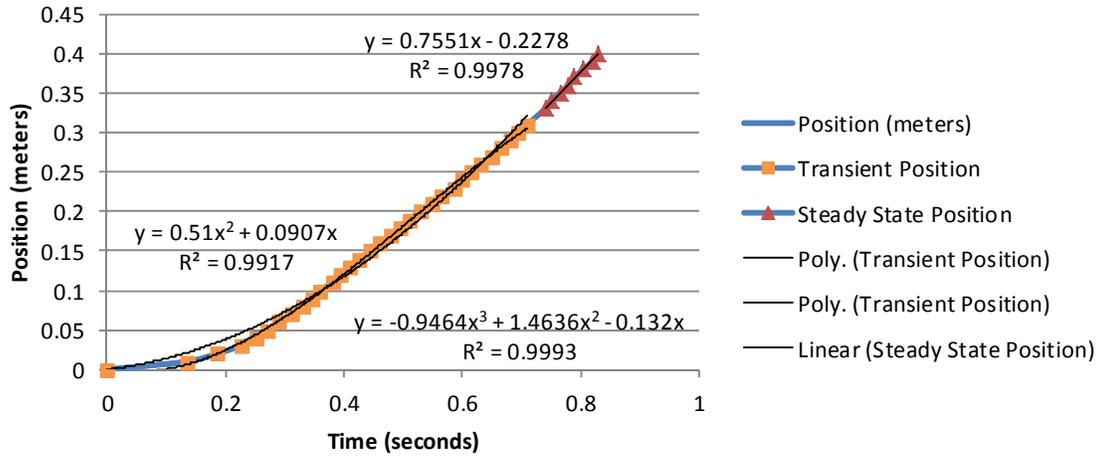
Figure 131 Frame position vs time at 6 Hz speed setting
