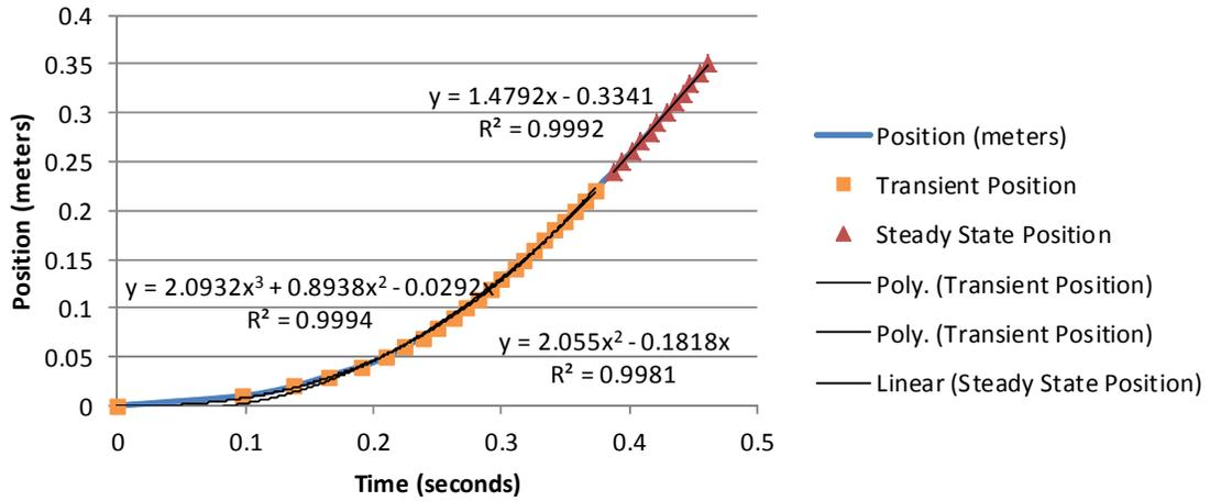
Figure 125 Frame position vs time at 9 Hz speed setting
