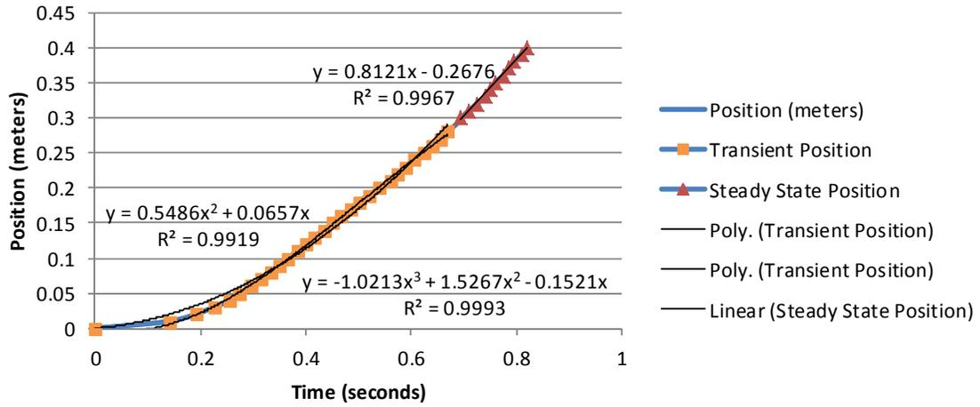
Figure 133 Frame position vs time at 7 Hz speed setting
