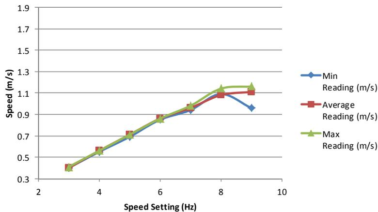
Figure 37 Frame developed steady state velocity in water
