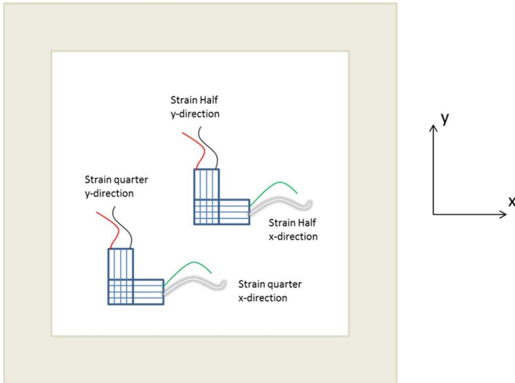
Figure 14 Strain gauge orientation
