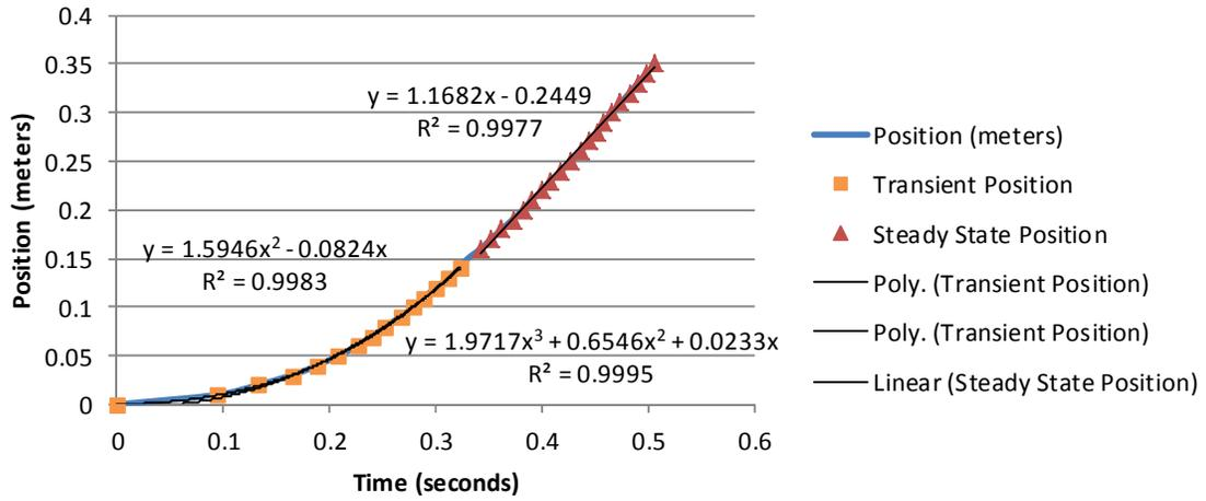
Figure 123 Frame position vs time at 8 Hz speed setting
