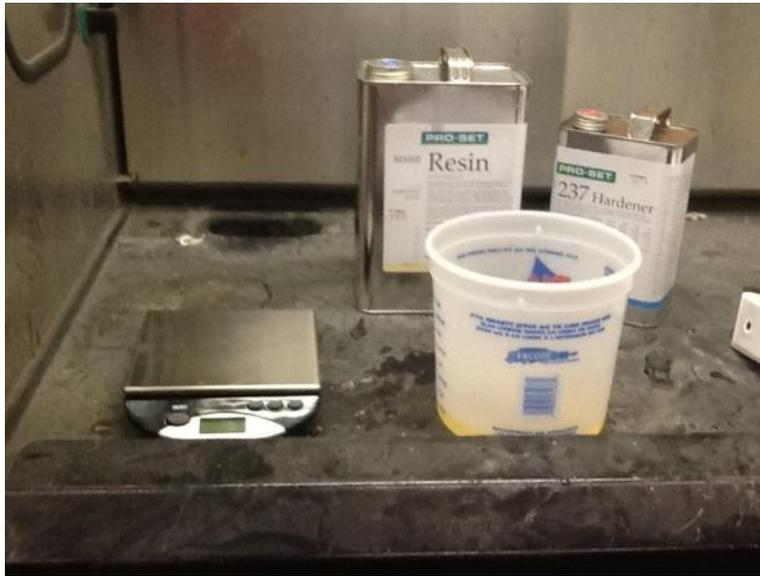
Figure 11 Resin/Hardener measuring by weight
