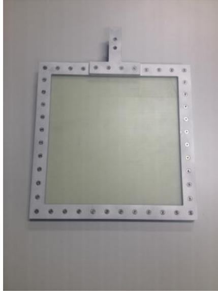
Figure 9 Front view of frame test piece with six-layer composite
