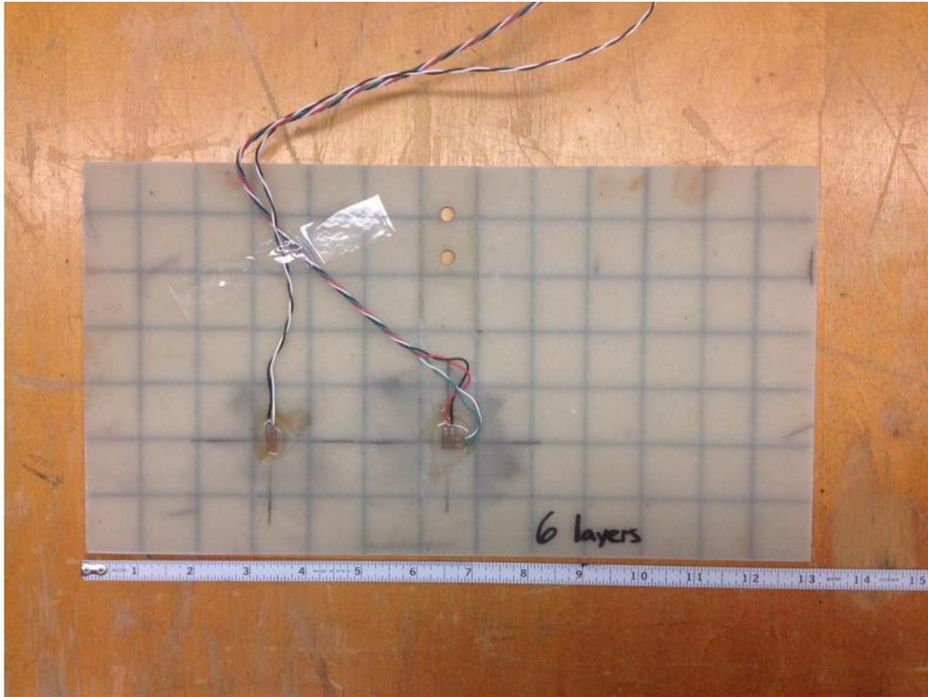
Figure 8 330x178 mm six-layer composite plate test piece
