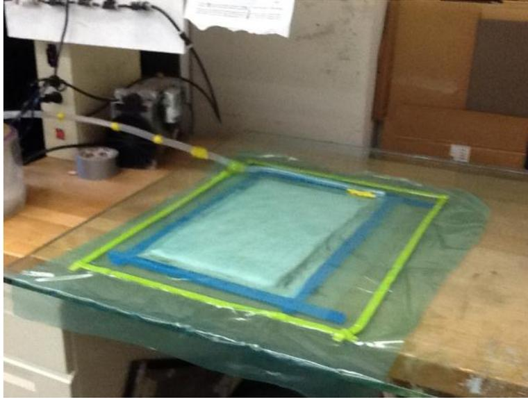
Figure 13 Vacuum set up over composite sample
