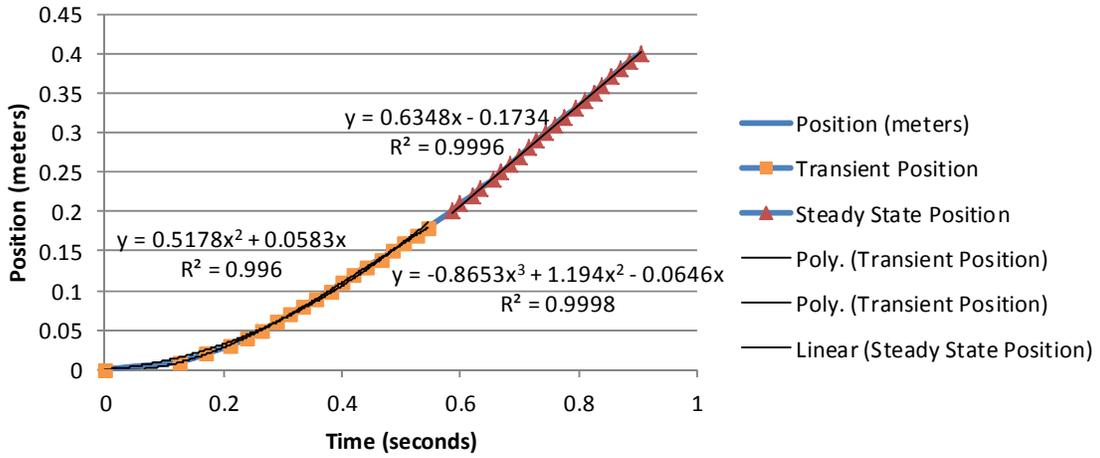
Figure 129 Frame position vs time at 5 Hz speed setting
