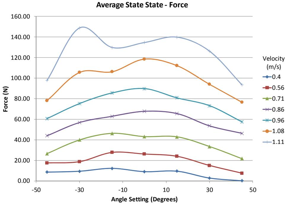
Figure 73 Framed composite average steady state force
