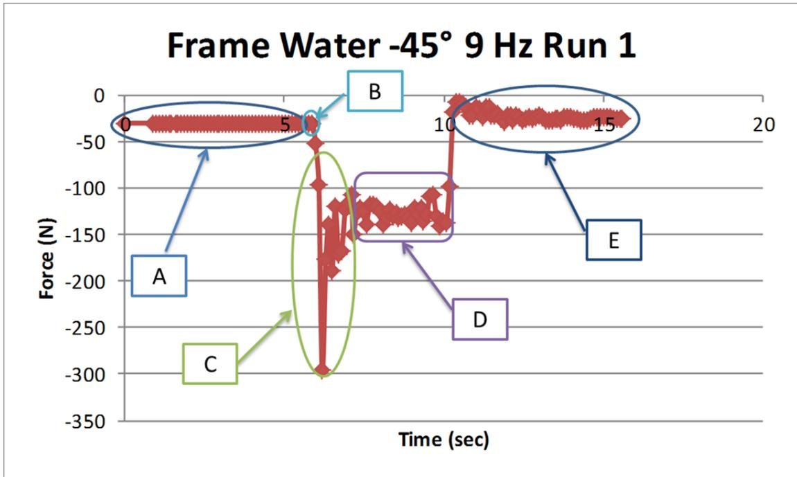
Figure 24 Nomenclature associated with data acquisition system (A) static force, (B) starting point where  $t=0$  and  $F=0$  once normalized, (C) transient zone, (D) steady state zone, and (E) post run static force
