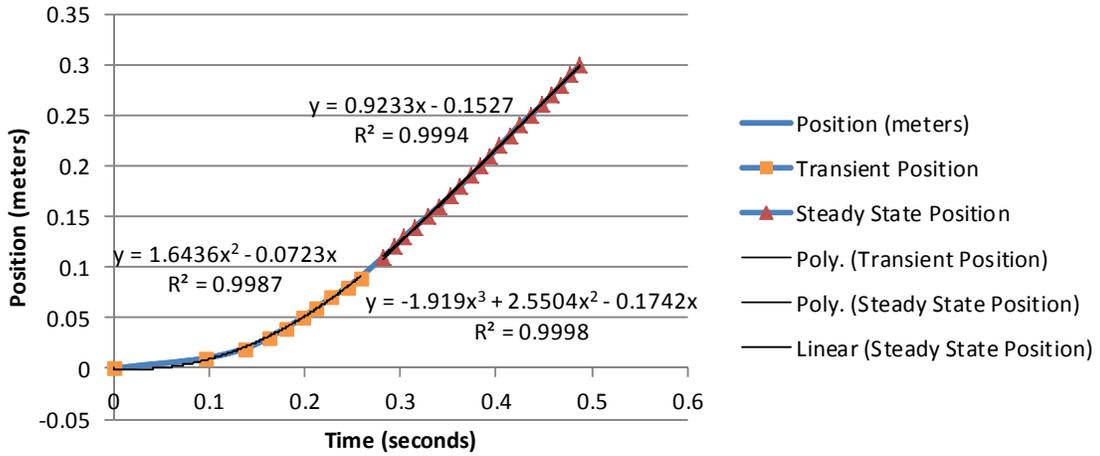
Figure 107 Aluminum sample position vs time at 6 Hz speed setting
