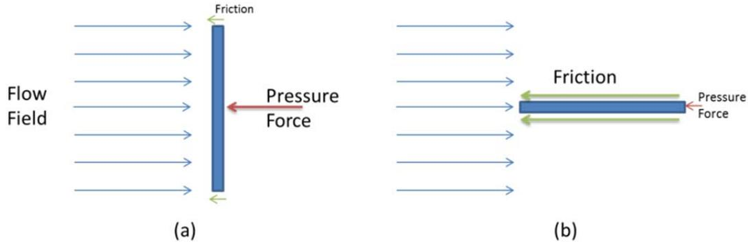
Figure 5 Body orientation influence on imparted fluid force
