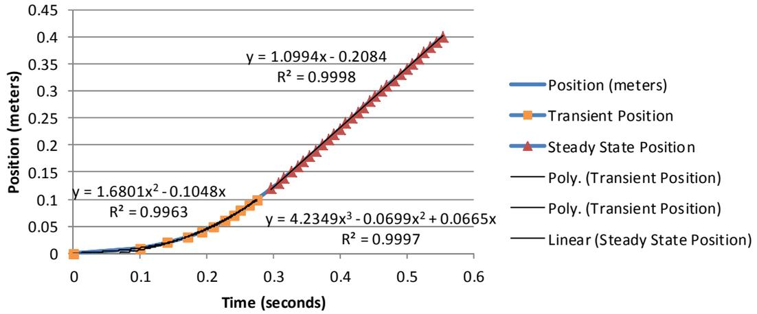
Figure 109 Aluminum sample position vs time at 7 Hz speed setting
