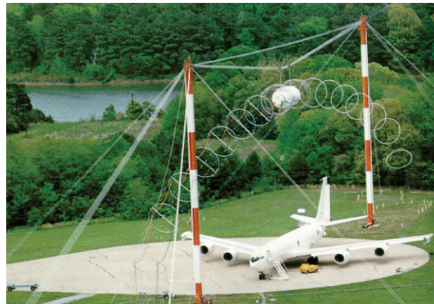
Figure 1: Horizontally Polarized Dipole EMP simulator previously utilizing the ML-5 pulser source.
