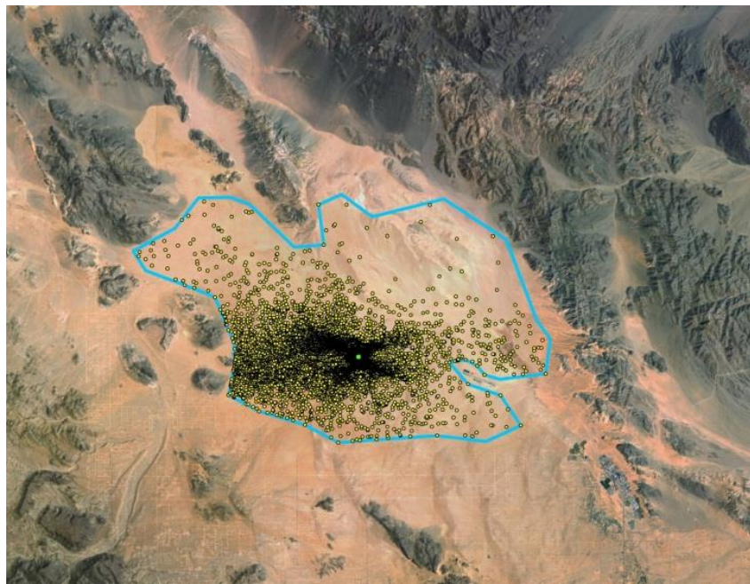
Figure 4. Data collection for the measurement footprint at the Marine Corps Air Ground Combat Center (MCAGC, light blue line). The green dot indicates the location of the EC tower. Yellow points represent individual 30-min flux values measured by the EC instrumentation between June 15, 2011 and June 15, 2012.
