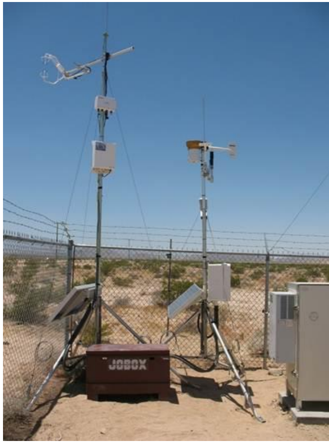
Figure 3. Photograph of the eddy covariance (EC) instrumentation at the Marine Corps Air Ground Combat Center (MCAGCC) near Twentynine Palms, California. The instrumentation was installed on June 15 2011. The rightmost tripod tower in the photograph is the 5-m tripod tower and contains the EC instrumentation. The leftmost tower in the photograph is the 3-m tripod tower and contains the meteorological instrumentation.
