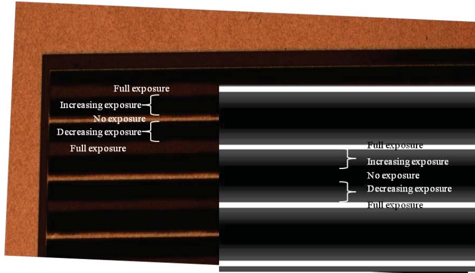
Figure 11. The results of etching of a 2D pyramid pattern into the silicon substrate, the image of the direct write pattern is on the right and the resulting etch into the silicon can be seen on the left.
