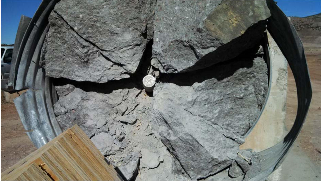
Fig. 14-50. Concrete target from Test 8, Design DTV-E-2.
