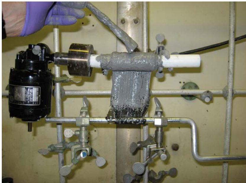
Fig. 5-7. Infiltration of braid with the epoxy-metal-powder slurry.
