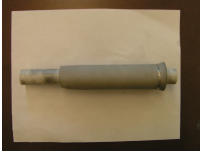
Fig. 4-6. CIP Hf/Al green construct approximately 1.5" OD x 1.0" ID x 6" L.
