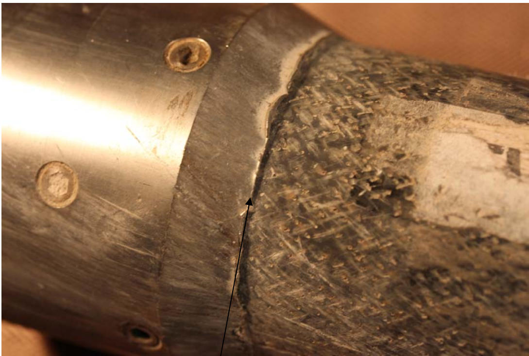
(a) Mark indicating axial compression of case within forward sleeve
