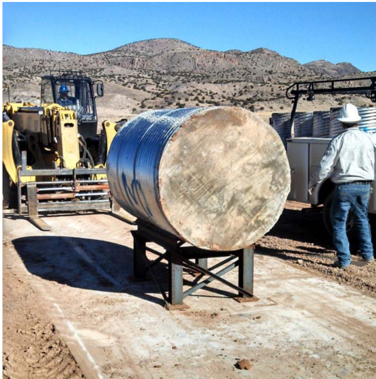
Fig. 14-11. Concrete target, 48 inches in diameter by 72 inches.
