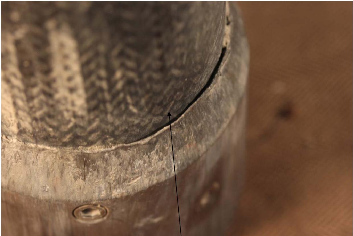
Damage to aft steel closure.
