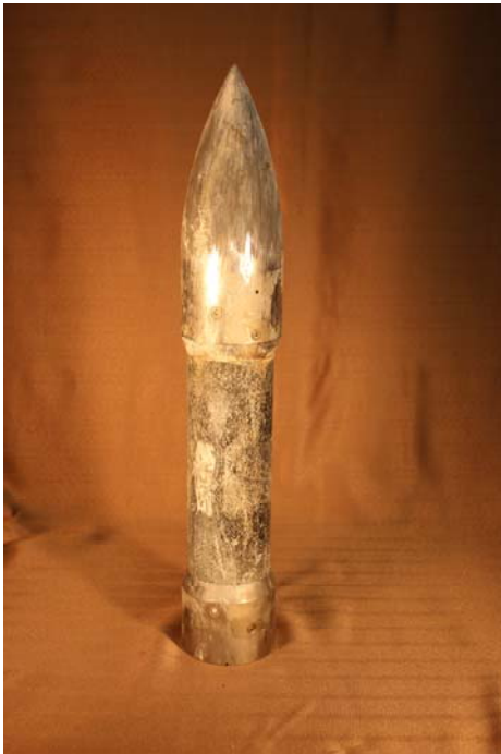
Fig. 14-35. Photographs of DTV-D-2 Penetrator from Test 5 at 0°, 90°, 180°, and 270°.
