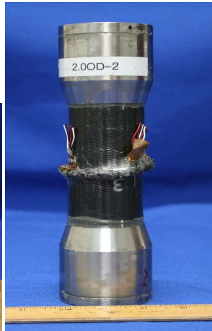
Fig. 9-17. Post-test photographs of 2.0-inch-diameter compression specimens.
