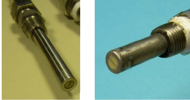
Fig. 6-62. Photographs of a new Nanmac thermocouple (left) and a resurfaced end (right).
