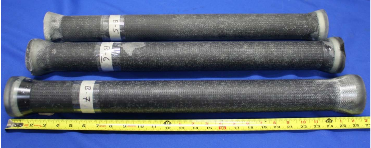
Fig. 9-31. Specimens for the flex-bend tests.
