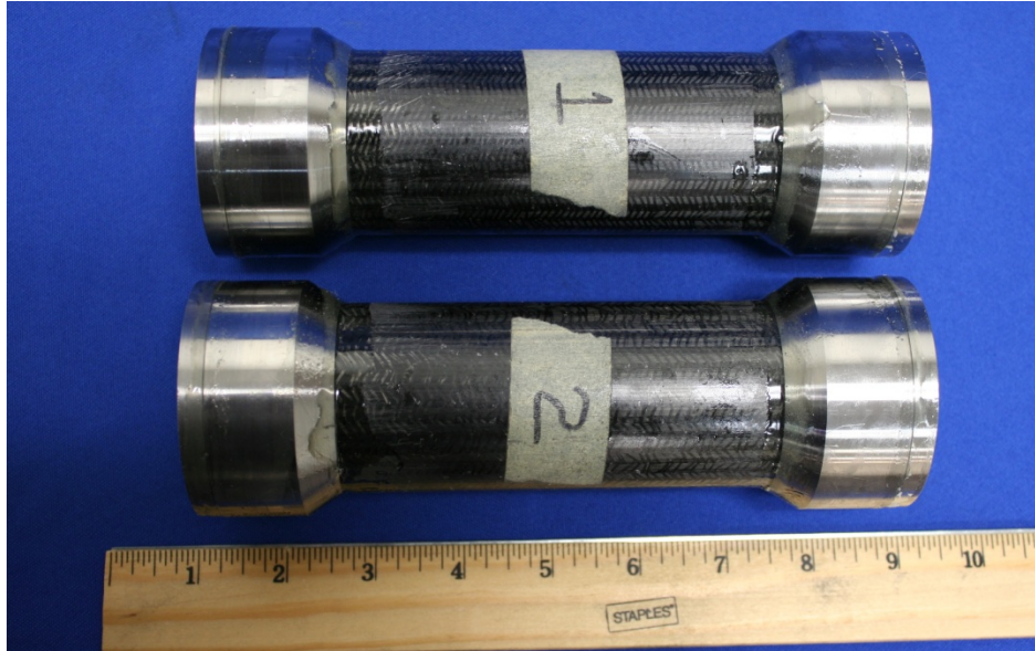
Fig. 9-12. Assembled compression test specimens.
