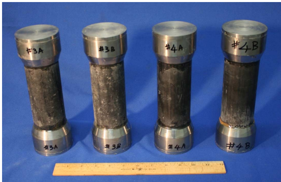
Fig. 9-24. Photograph of 2.5-inch-diameter compression specimens.
