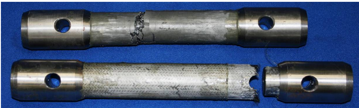
Fig. 2-17. Fracture of tensile-test cylinders of Al-Hf-W-Ep (top) and Al-W-Ep (bottom).
