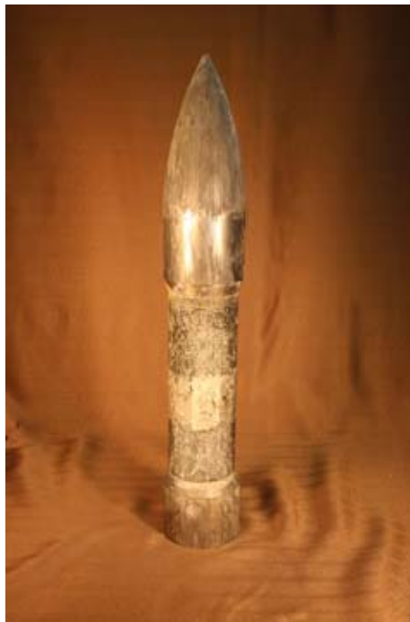
Fig. 14-30. Photographs of DTV-A-1 Penetrator from Test 4 at 0°, 90°, 180°, and 270°.
