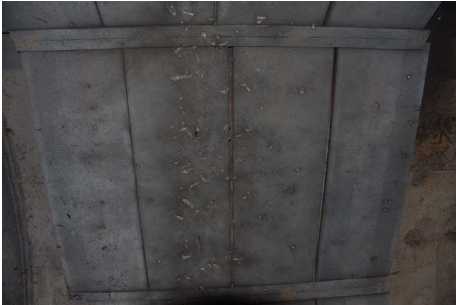
Fig. 10-16. Fragment damage to armor plating.
