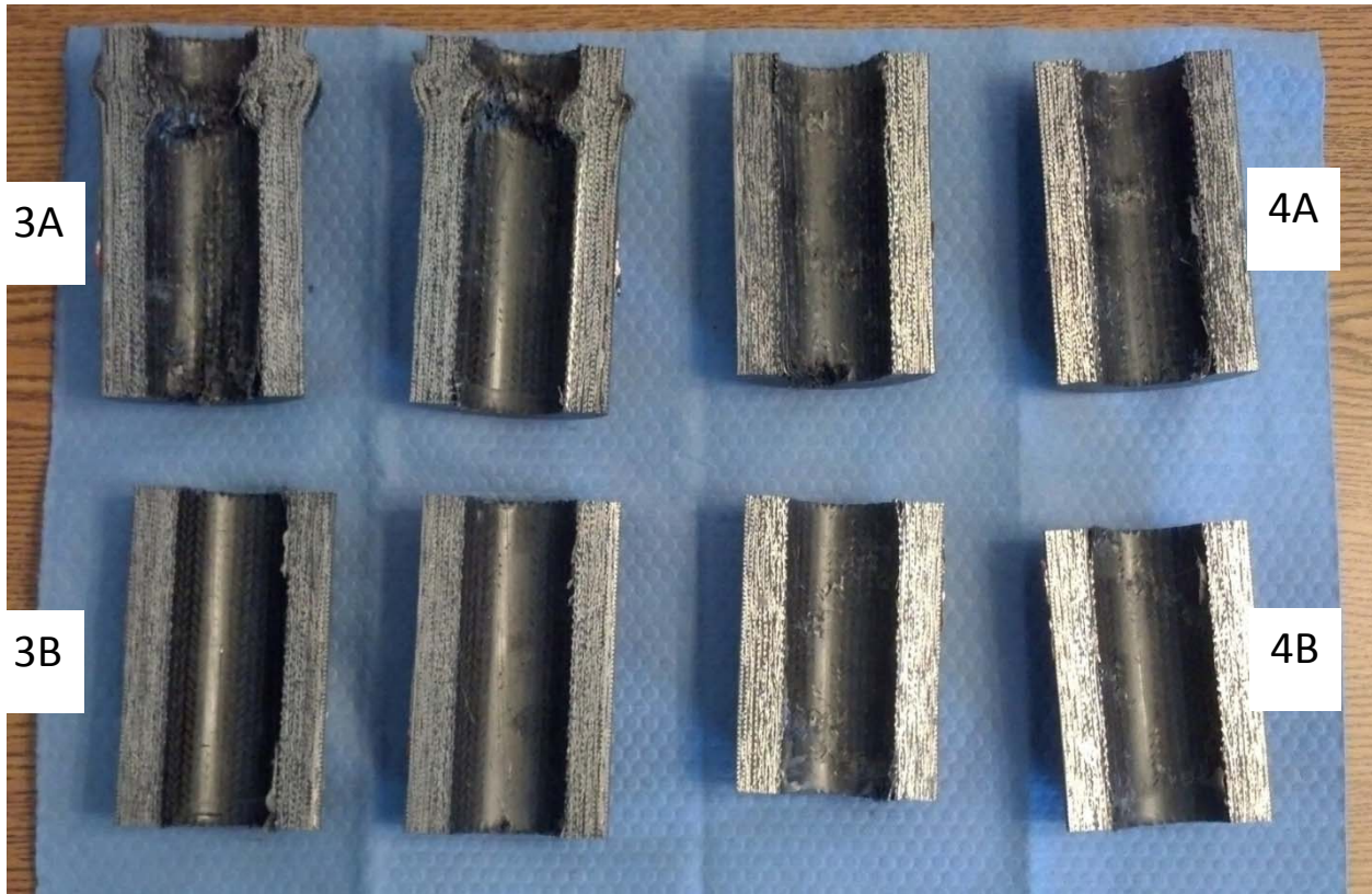
Fig. 9-28. Post-test photograph of sectioned 2.5-inch-diameter compression specimens.
