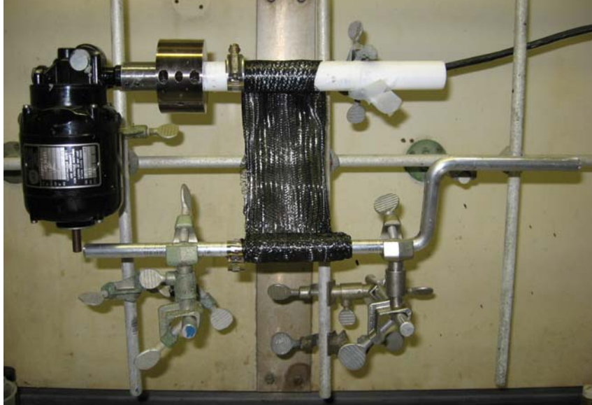
Fig. 5-6. Mounting of braid in fixture.
