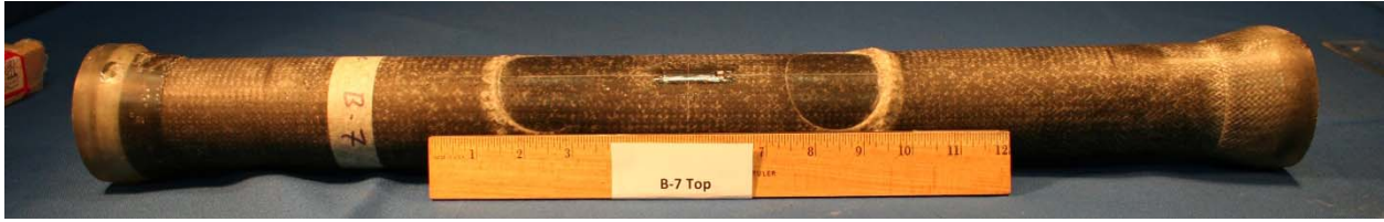
Post flex test number 3, specimen B-7, top (load) view
