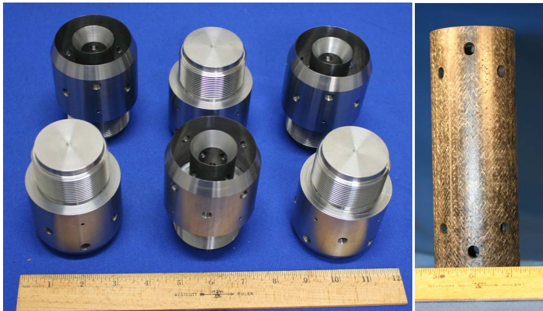
Fig. 12-29. Compression/tension specimen hardware.
