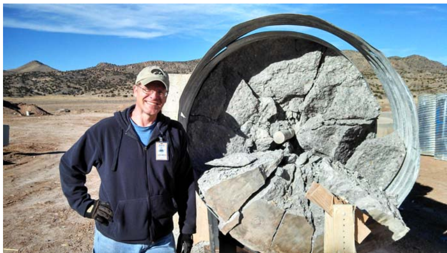
Fig. 14-15. Concrete target from Test 1, Design DTV-E-1, EMRTC technician for size reference.
