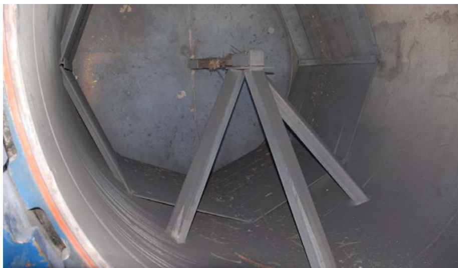
Fig. 10-14. Steel tripod mounting the test charge between wooden supports oriented coaxially within the chamber.
