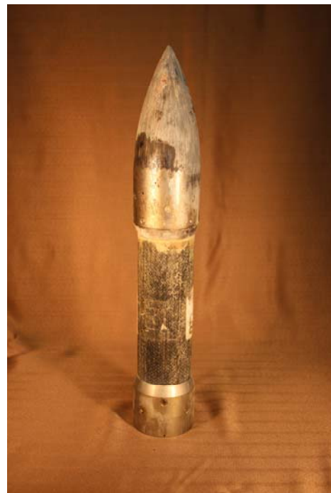
Figure 14-45. Photographs of DTV-D-4 Penetrator from Test 7 at 0°, 90°, 180°, and 270°.
