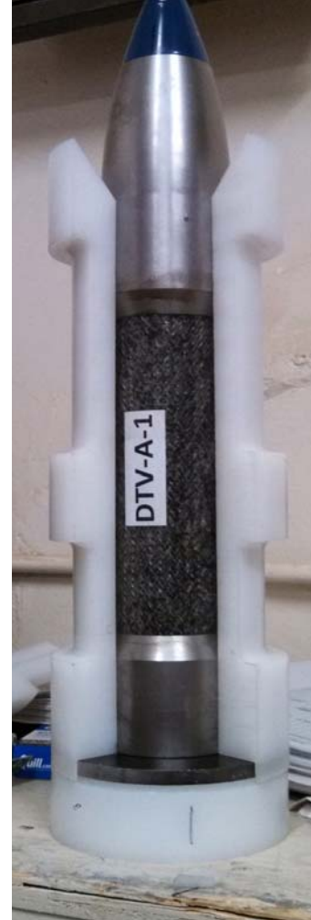
(c) Design-3, internal step removed with cylindrical channels along the length
