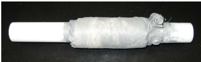
Fig. 5-11. Specimen after dismounting from fixture.
