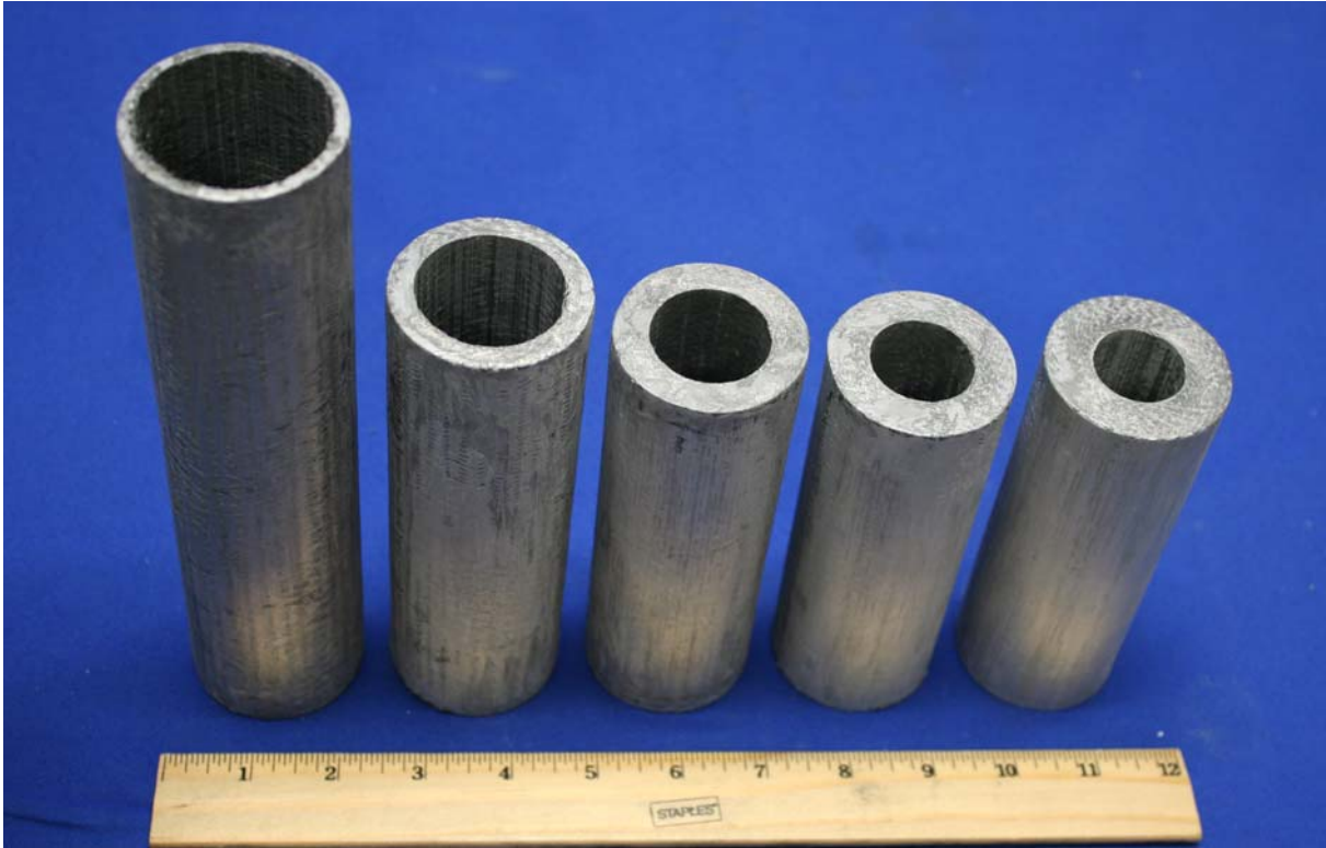
Fig. 10-2. RMS specimens for the M/C blast study, with M/C 's (from left to right) of 1, 3, 6, 9, and 12.
