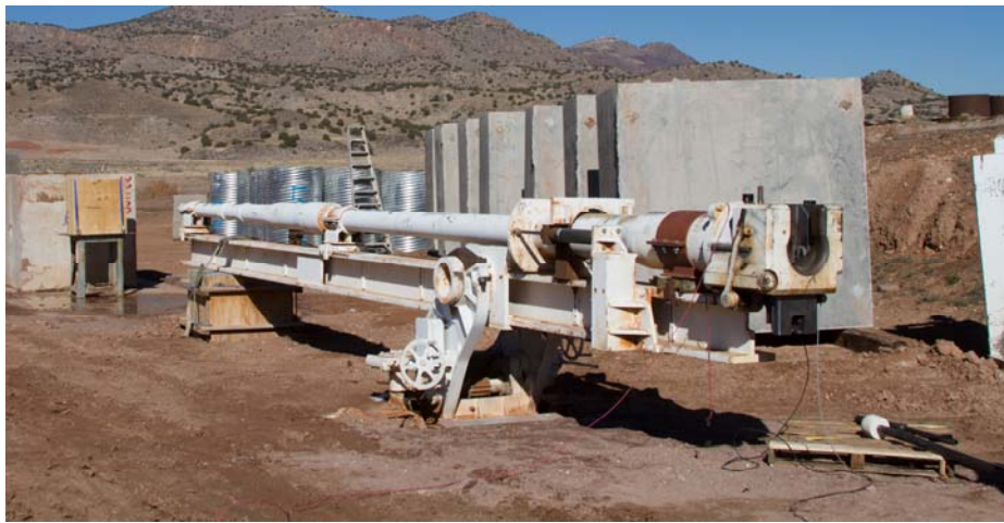
Fig. 14-9. EMRTC 5-inch-Diameter Smoothbore Powder Gun.
