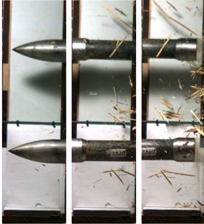
Fig. 14-42. Images from orthogonal video of Test Number 7, Design DTV-D-4.
