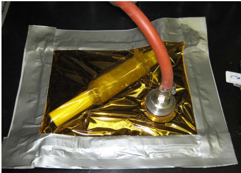
Fig. 5-12. Specimen during vacuum curing.
