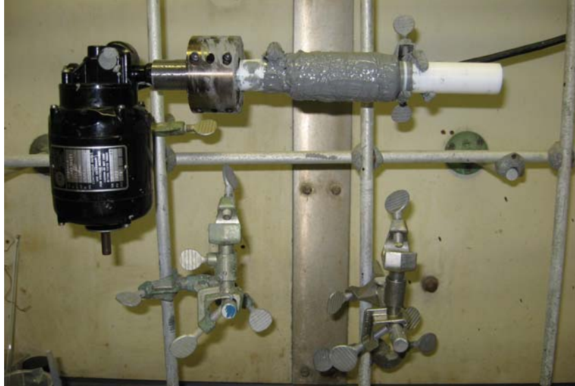
Fig. 5-8. Specimen after infiltration with slurry.
