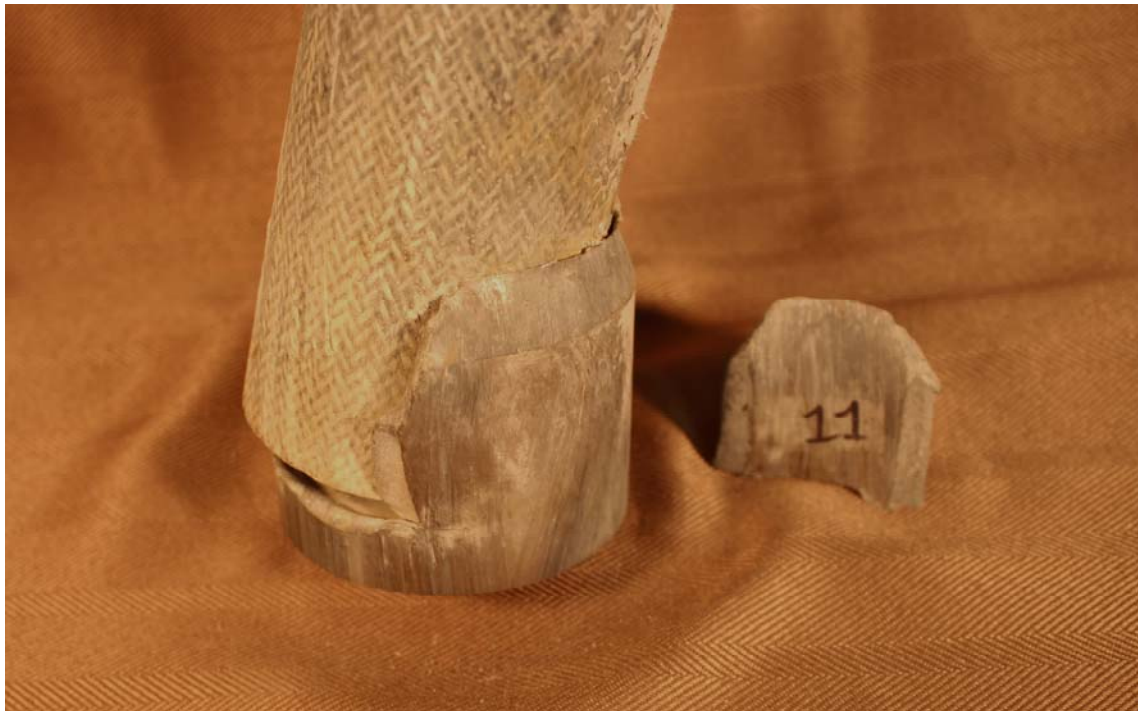
Fig. 14-69. Damage to the DTV-B-2 Penetrator from Test 11.
