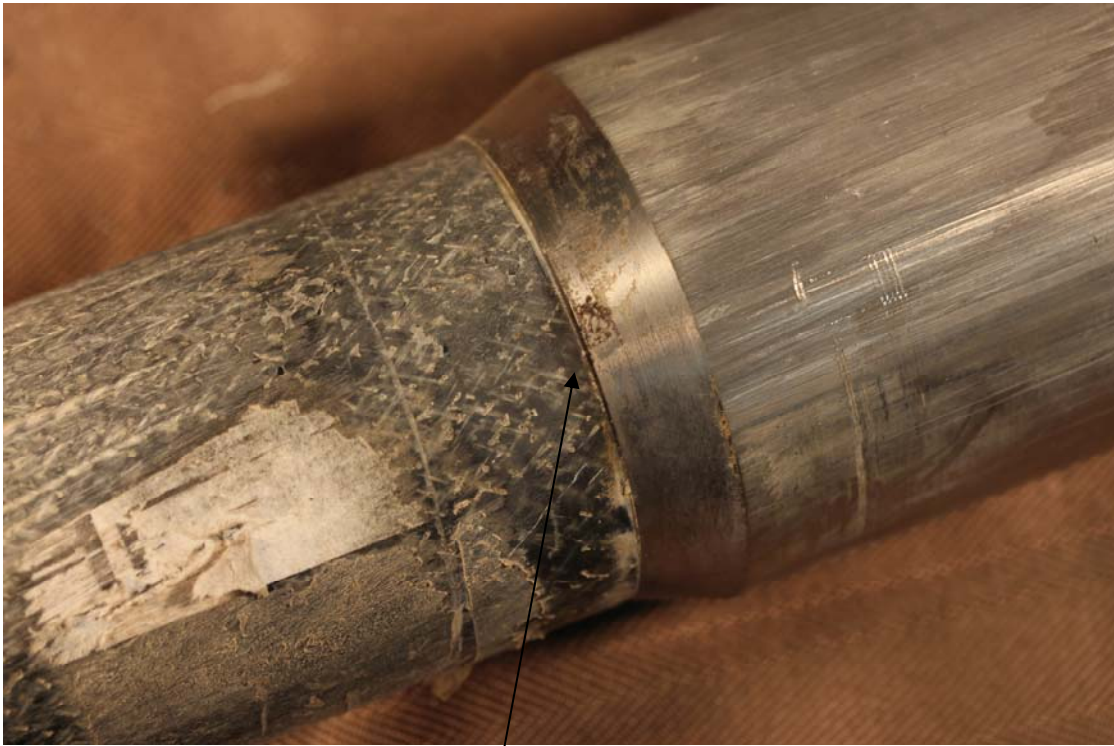
(a) Mark indicating axial compression of case within forward sleeve
