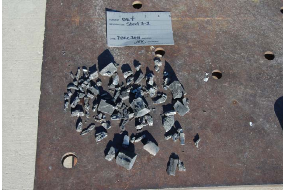
Fig. 10-17. Recovered metal fragments from end caps and casing. The blast test parameters are summarized in Table 10-4.
