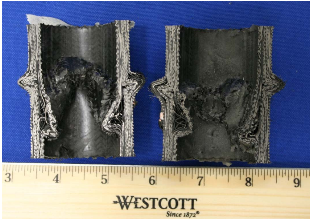
Fig. 9-20. Photograph of sectioned 2.0-inch-diameter specimen FEB13-2.
