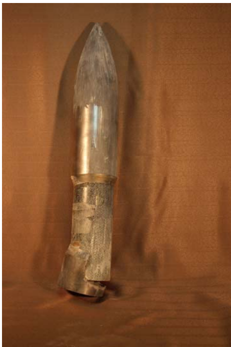
Fig. 14-68. Photographs of DTV-B-2 Penetrator from Test 11 at 0°, 90°, 180°, and 270°.
