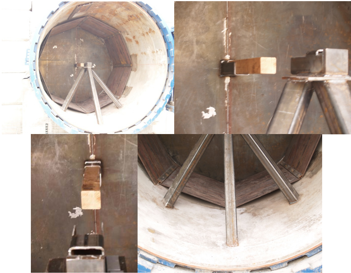
Fig. 10-8. Test stand construction consisted of a steel tripod and bracket on bulkhead.
