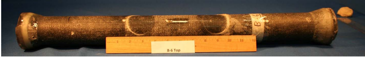
Post flex test number 2, specimen B-6, top (load) view
