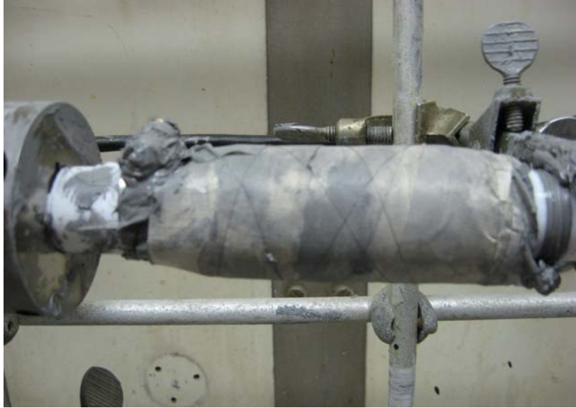
Fig. 5-10. Specimen after wrapping and binding with tungsten wire.
