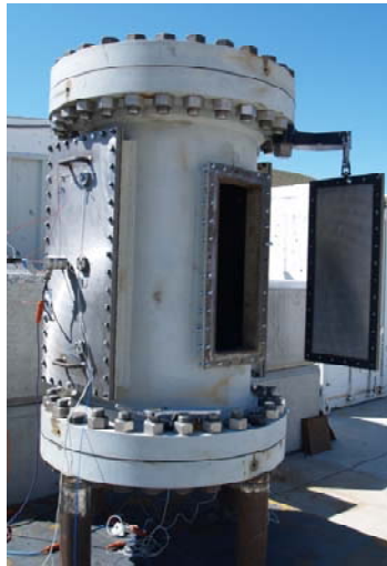
Fig. 6-58. Exterior of ATK's explosive chamber showing the front access door and the side panels.
