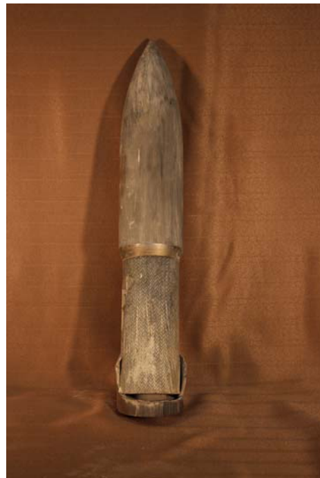
Fig. 14-68. Photographs of DTV-B-2 Penetrator from Test 11 at 0°, 90°, 180°, and 270°.
