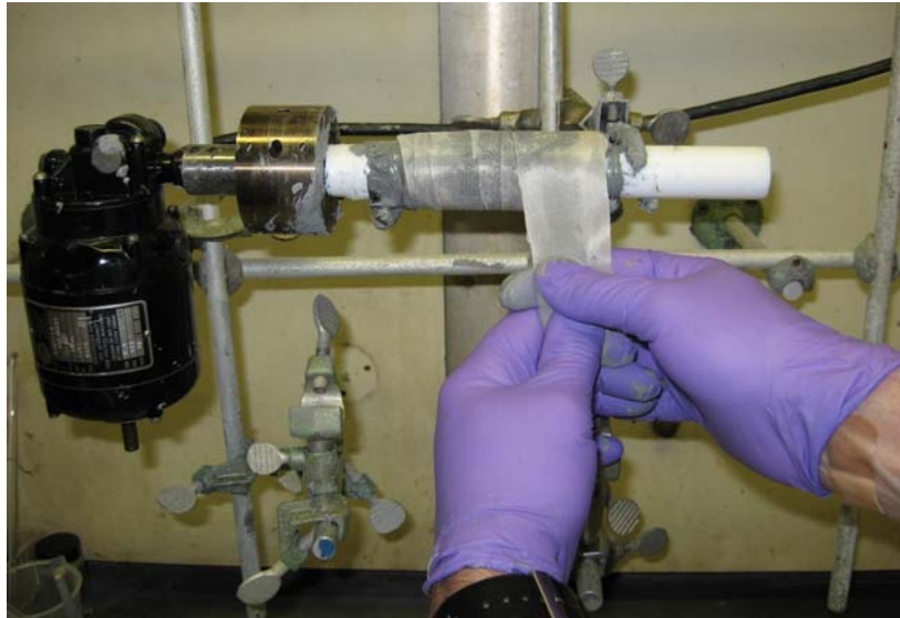
Fig. 5-9. Wrapping specimen with glass mesh.
