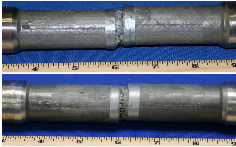
Fig. 2-15. Fracture of tensile specimen with groove in gage region showing the tungsten wires in the inner layers remained intact. Al-W-Ep (top) and Al-Hf-W-Ep (bottom).
