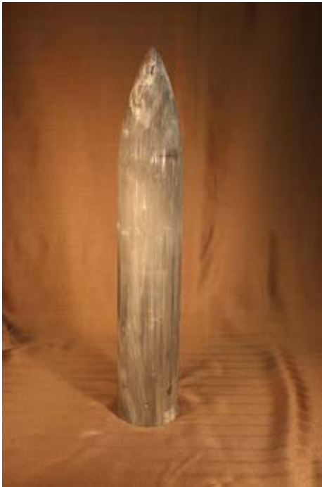
Fig. 14-78. Photographs of DTV-F-2 Penetrator from Test 13 at 0°, 90°, 180°, and 270°.
