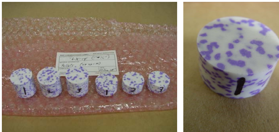
Fig. 6-57. Pressed LX-14 charges with L/D=1 and L/D=0.5.
