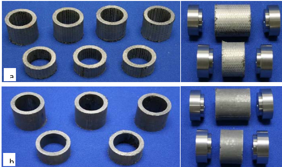
Fig. 2-12. Blast test specimens: a) Al-W-EP, and b) Al-Hf-W-Ep. Specimen length for small chamber tests: ATK: 1.25"; UIUC: 0.75" and 1.25"; and ARA: 1" (fragmentation test) and 3" (fully closed chamber test).
