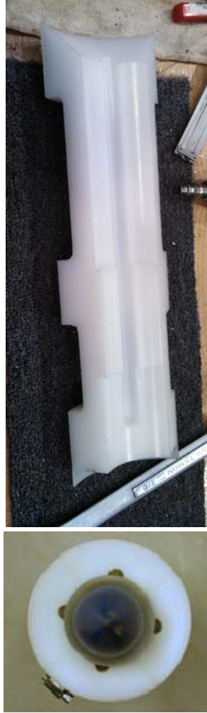
(b) Design-2, stepped internal surface matching outside diameter of composite case with cylindrical channels along the length
