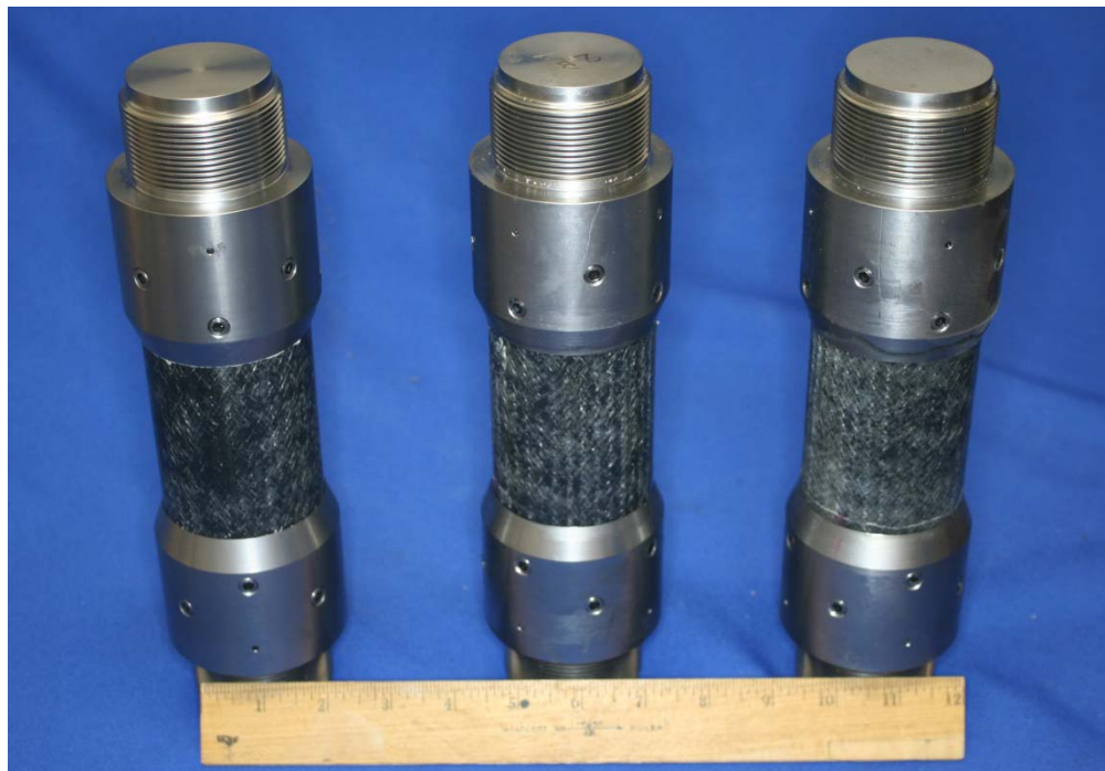
Fig. 12-30. Assembled compression/tension specimen.
