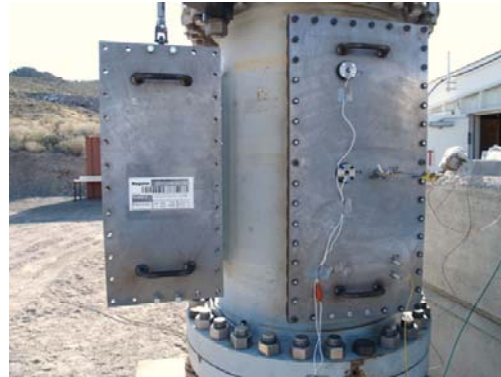
Fig. 6-58. Exterior of ATK's explosive chamber showing the front access door and the side panels.
