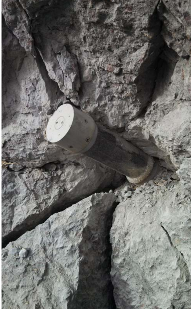
Fig. 14-39. Concrete target from Test 6, Design DTV-D-3.
