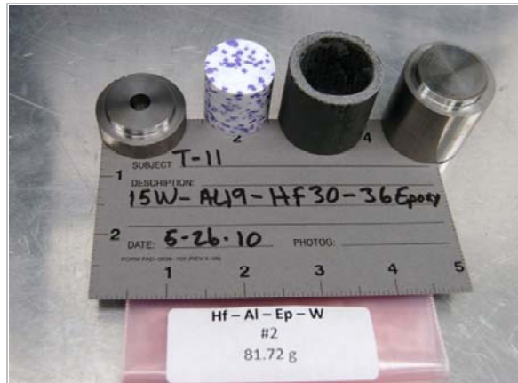
Fig. 6-66. Test article prior to assembly. From left to right: the detonator housing confinement, LX-14 explosive charge, RMS case, and end confinement.
