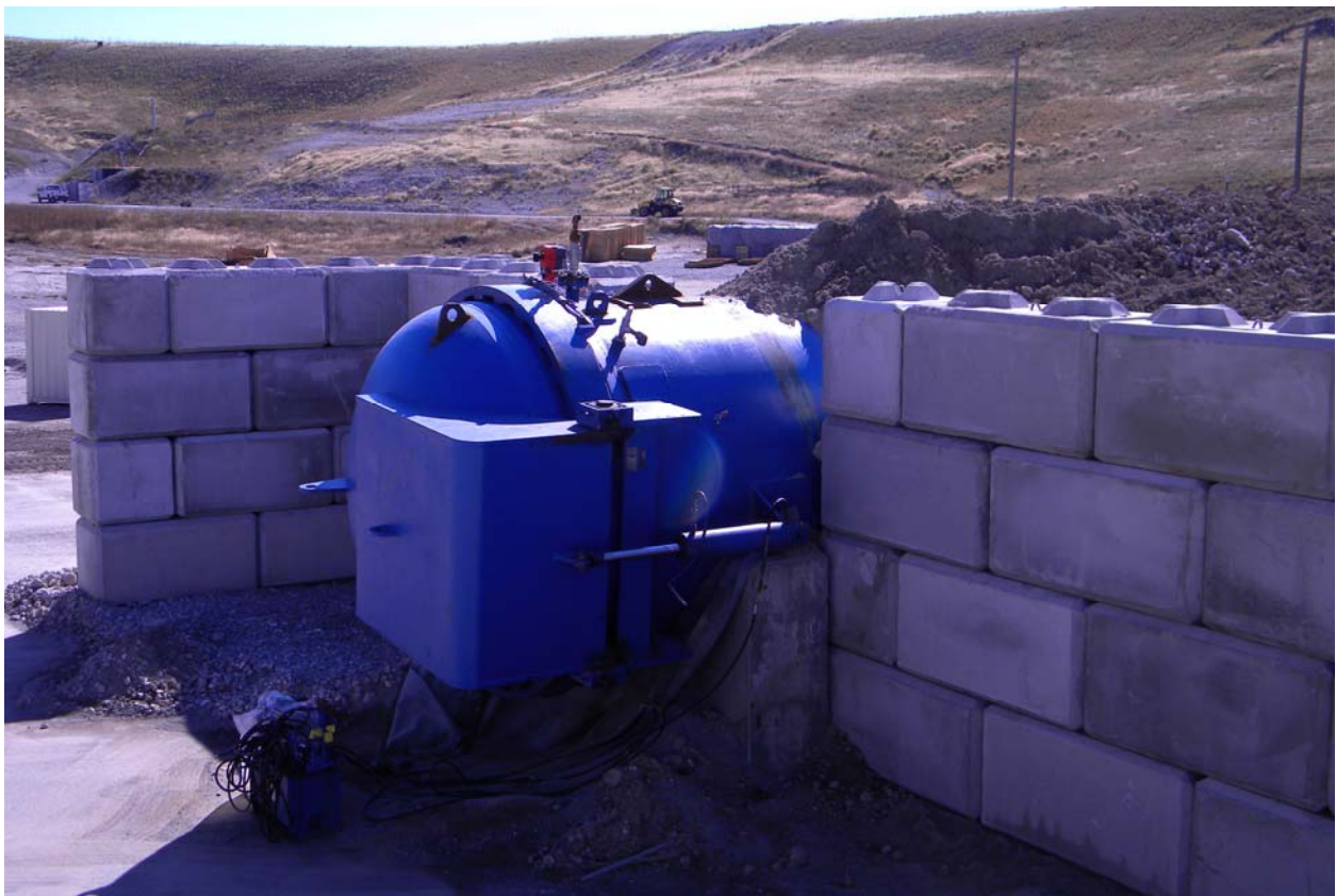
Fig. 10-5. ATK test site showing emplaced blast chamber to be used for M/C tests.
