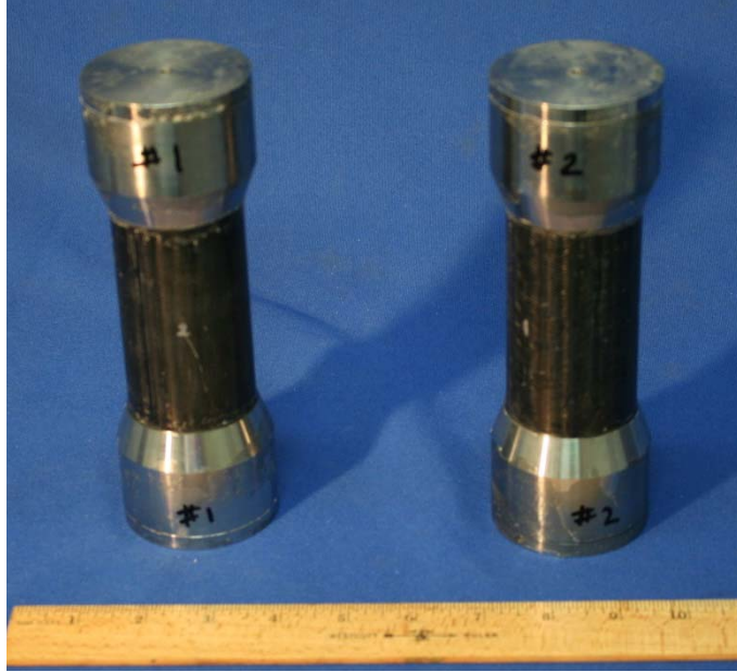
Fig. 9-15. The 2.0-inch-diameter compression specimens.
