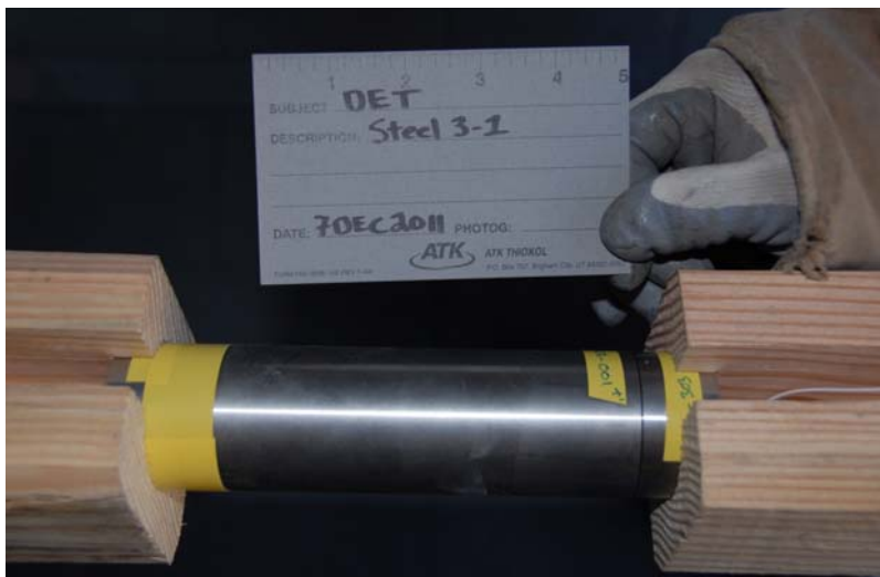
Fig. 10-13. Steel-cased explosive charge mounted between wooden supports.
