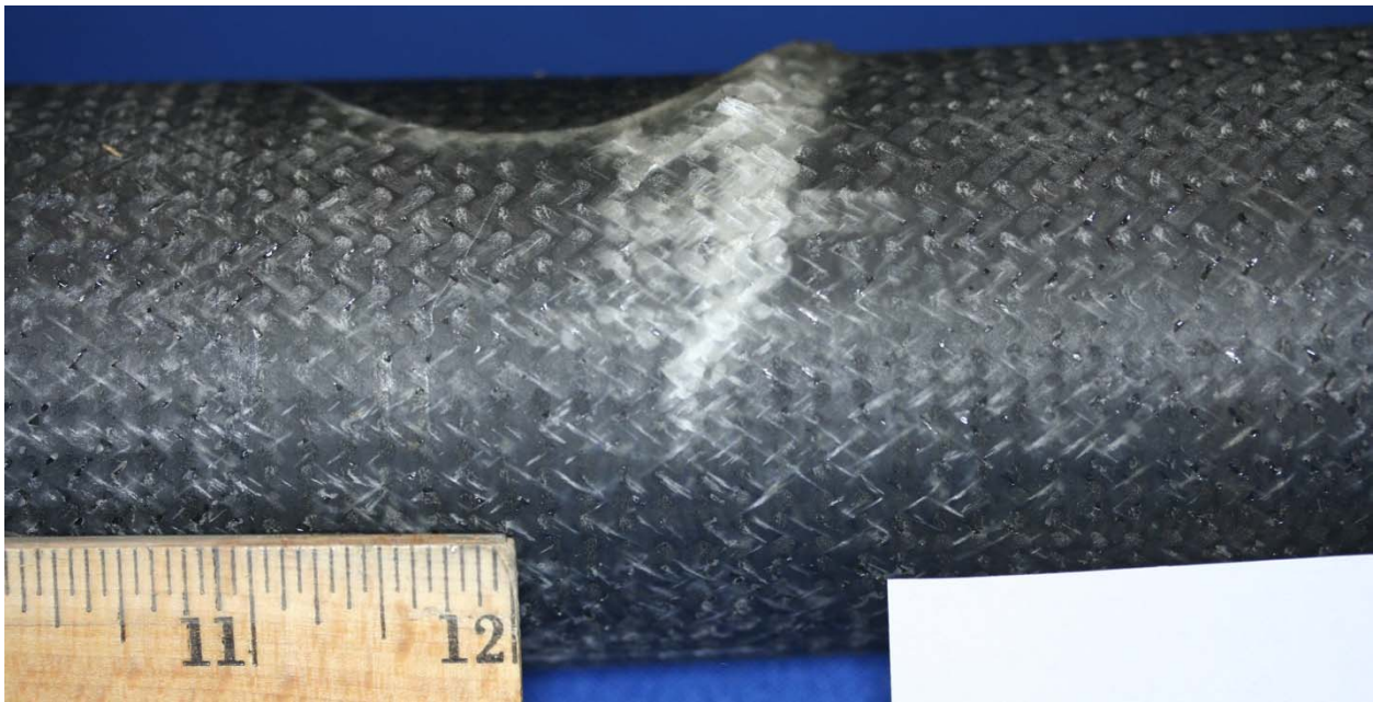
Post flex test number 3, specimen B-7, shear band from load applicator Fig. 9-38. Post-test photographs of flex test number 3, specimen B-7.
