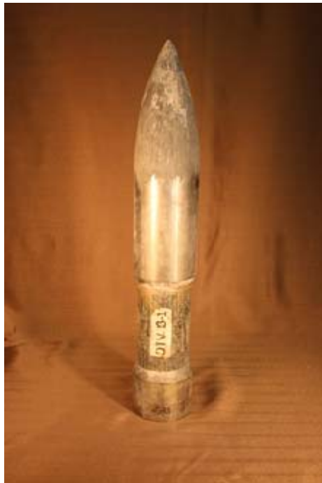
Fig. 14-21. Photographs of DTV-B-1 Penetrator from Test 2 at 0°, 90°, 180°, and 270°.
