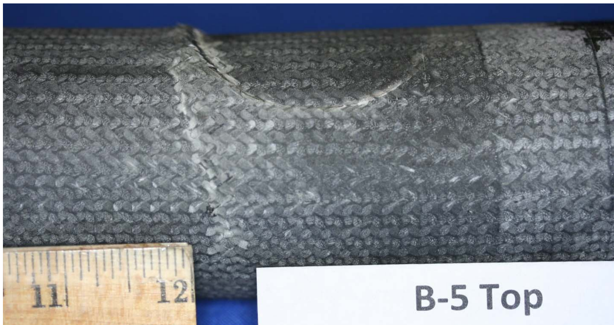
Post flex test number 1, specimen B-5, shear band from load applicator
