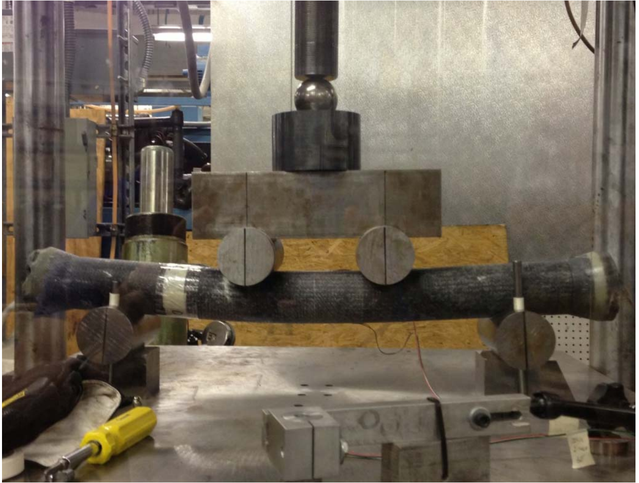
Fig. 9-33. Flex test during loading.
