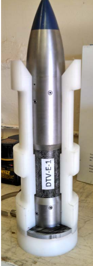
(a) Design-1, stepped internal surface matching outside diameter of composite case
