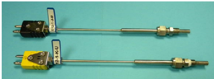
Fig. 6-61. Nanmac high-temperature fast-response thermocouples.
