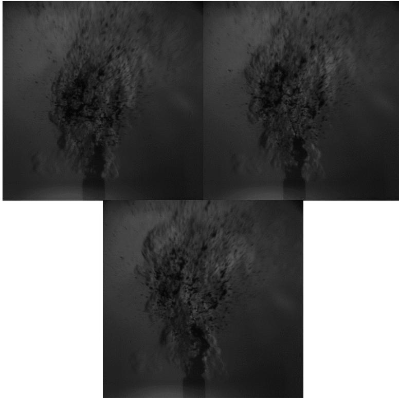
**Figure 6:** High-speed images of the helium jet with water droplets, recorded 0.0004 seconds apart. The images show the breakup and dispersion of the water jet and the interactions with the turbulent structure of the jet.
