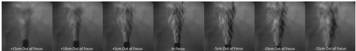
**Figure 4:** Focusing schlieren images demonstrating the focusing effect as the helium jet is transitioned along the optical axis. The position of best focus is in the middle of the compilation.
