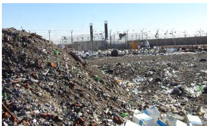
Photo 3 - Open-Air Burn Pit at Shindand Airbase, with Unused Afghan-Operated Incinerators in Background
