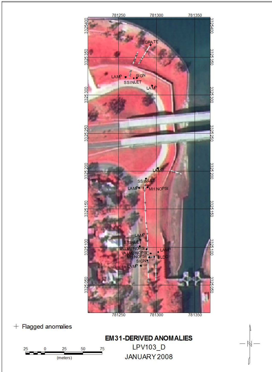
Figure 21. Anomalies interpreted from EM31 survey, LPV103_D.
