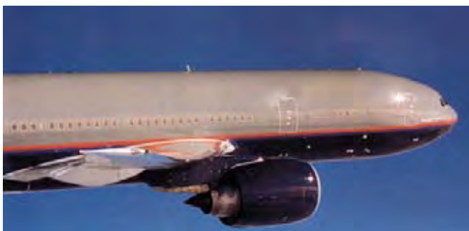
This commercial jet plane incorporates a supercritical wing design, which improves lift, resulting in better takeoff and landing performance. (NASA photo)
