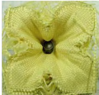
Right: Kevlar fabric stops a bullet. (Army photo)
