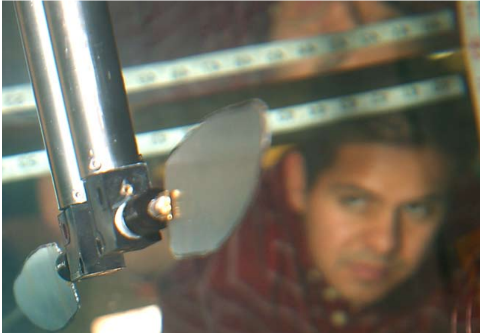
Testing a wing model in a water channel. (NMSU photo)
