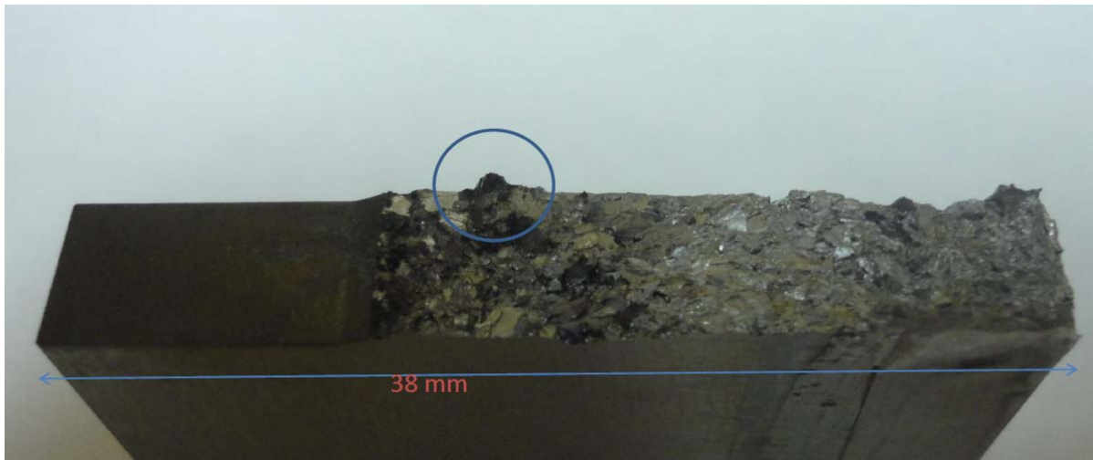
Figure 1: Crack surface on specimen 4A showing significant 1.5 mm asperity at a crack length of about 13-15 mm.
