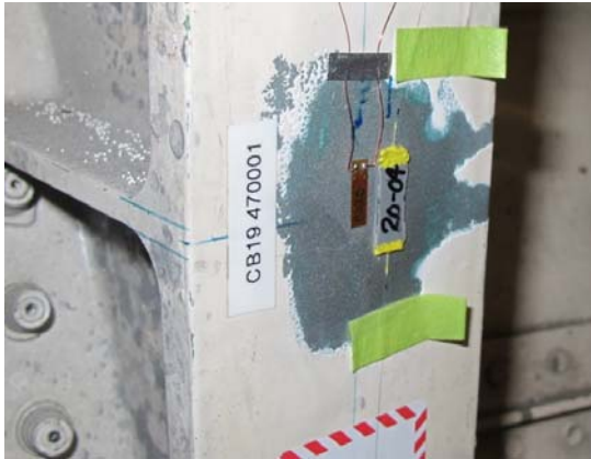
Figure 3: FBG sensor (labelled 20-04) collocated with conventional strain gauge foil on FINAL CB19 Y470.5 bulkhead.
