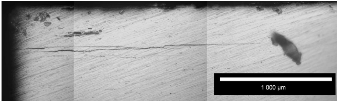
Figure 5: Optical micrograph of a path of intergranular corrosion in 7075-T6.
