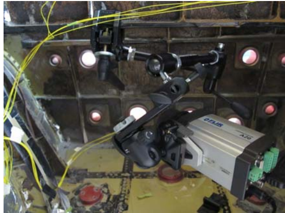
Figure 4: DSTO's portable TSA capability showing IR camera mounted to test article and focussed on highly loaded bulkhead region coated in primer.
