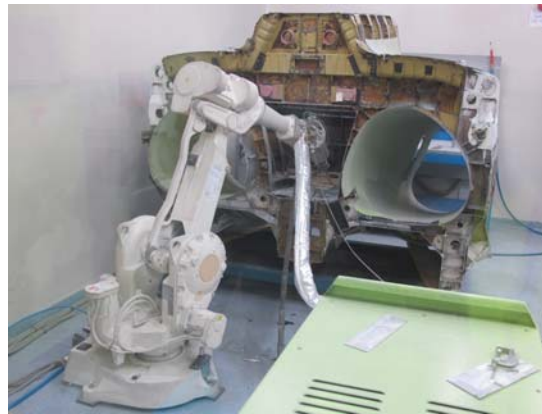
Figure 2: Robotic SPD application to the FINAL CB19 test article at Rosebank Engineering facility.
