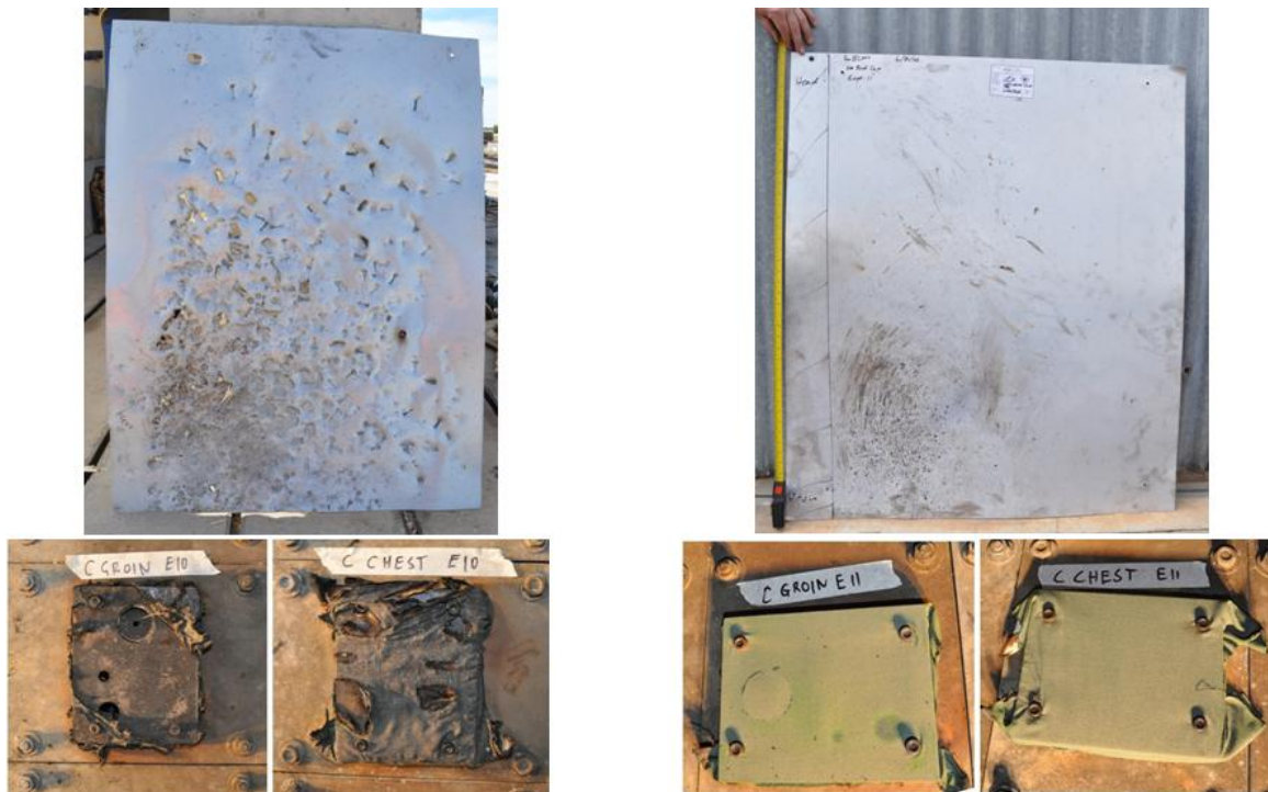
Figure 18: Effect of storage tube confinement on ejecta damage. LHS images: 3xBCM with end-cap (Experiment 10). RHS Images: 3xBCM no end-cap (Experiment 11).
