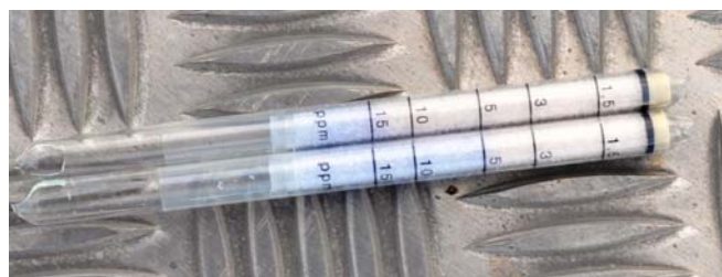
Figure 40: Drager tubes showing the presence of HF inside the trials structure after Experiment 6.
