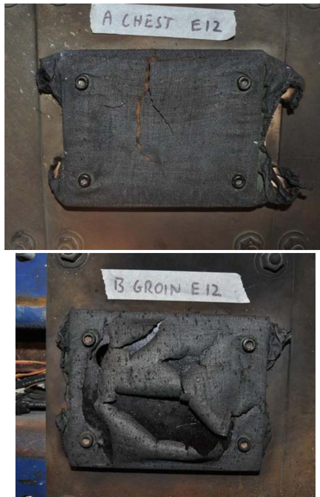
Figure 13: Burn damage sustained by the clothing of Person B groin and Person A chest for Experiment 12
