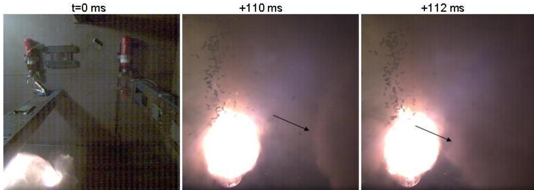
Figure 32: Camera images of Experiment 5 showing end-cap failure, subsequent propellant ejection and then suppressant plume from AFESS discharge (leading front of plume shown with arrows)
