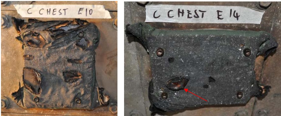
Figure 23: Chest of Person C showing, on the LHS, extensive ejecta damage (Experiment 10) and, on the RHS, exposure of the copper disc (buckled by ejecta impact) owing to ejecta strike during Experiment 14.
